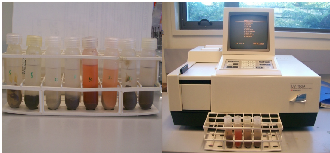
Figure 7.1: DHA samples and measurements using spectrophotometer.
