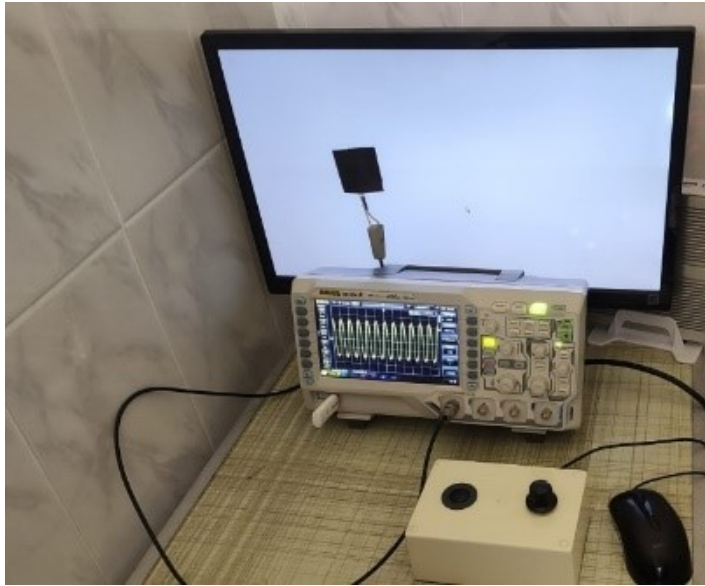
Figure 3.4: Photocell with a linear light-signal characteristic connected to an oscilloscope.
