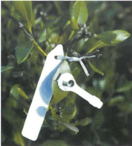
Plate 2.16 Dark-adaptation of an Avicennia marina subsp. australasica leaf in the field using a Walz darkening clip.
