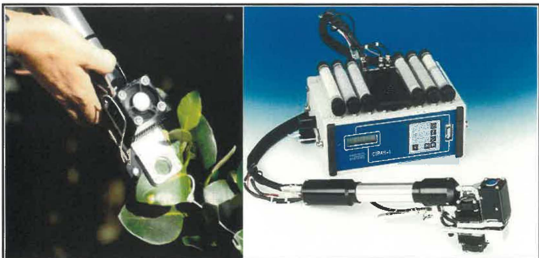
Plate 2.15 Left: The Parkinson Leaf Cuvette and measurement of leaf photosynthesis and transpiration in Avicennia marina subsp. australasica . (Photo: T.G.A. Green, 2002), Right: The CIRAS-1 Differential CO 2 /H 2 O Infra-Red Gas Analyser and Parkinson Leaf Cuvette. (Photo: PP-Systems, UK).
