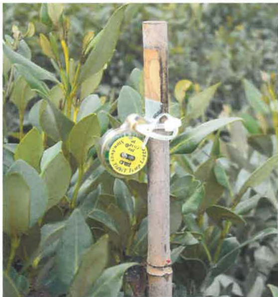
Plate 2.14 An unscreened Hobo StowAway TidbiT temperature logger attached in the upper canopy (approximately 1.5 m above the substrate) of Avicennia marina subsp. australasica plants, Ohiwa Harbour, Bay of Plenty. (Photo: C.Beard, July 2002)
