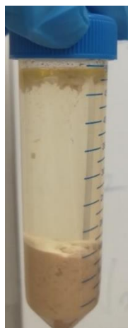
Figure 4.5: Centrifuged rendered fish in tube
