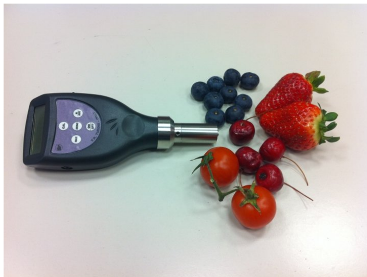
Figure 5.11: Turoi 53215BE, Non-destructive measurement of the firmness of soft fruit
