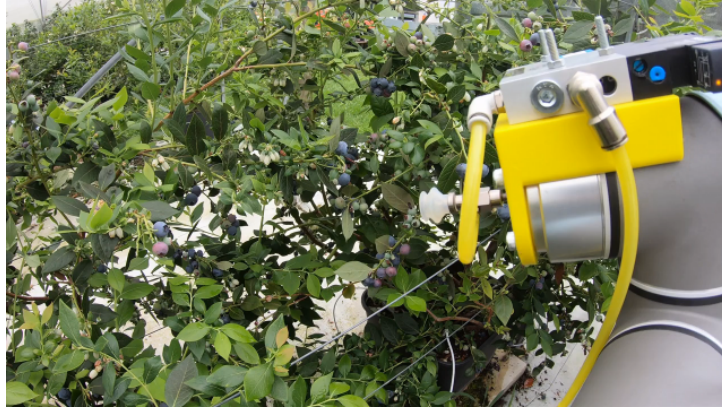
Figure 3.9: vacuum suction with silicon cup to detach berry
