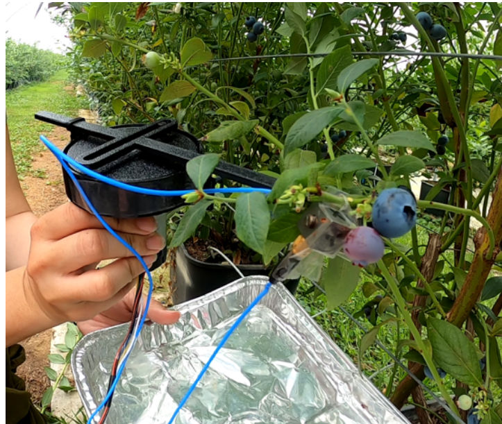
Figure 3.12: Reciprocating movements on berry cluster with a cam yoke shaking device.
