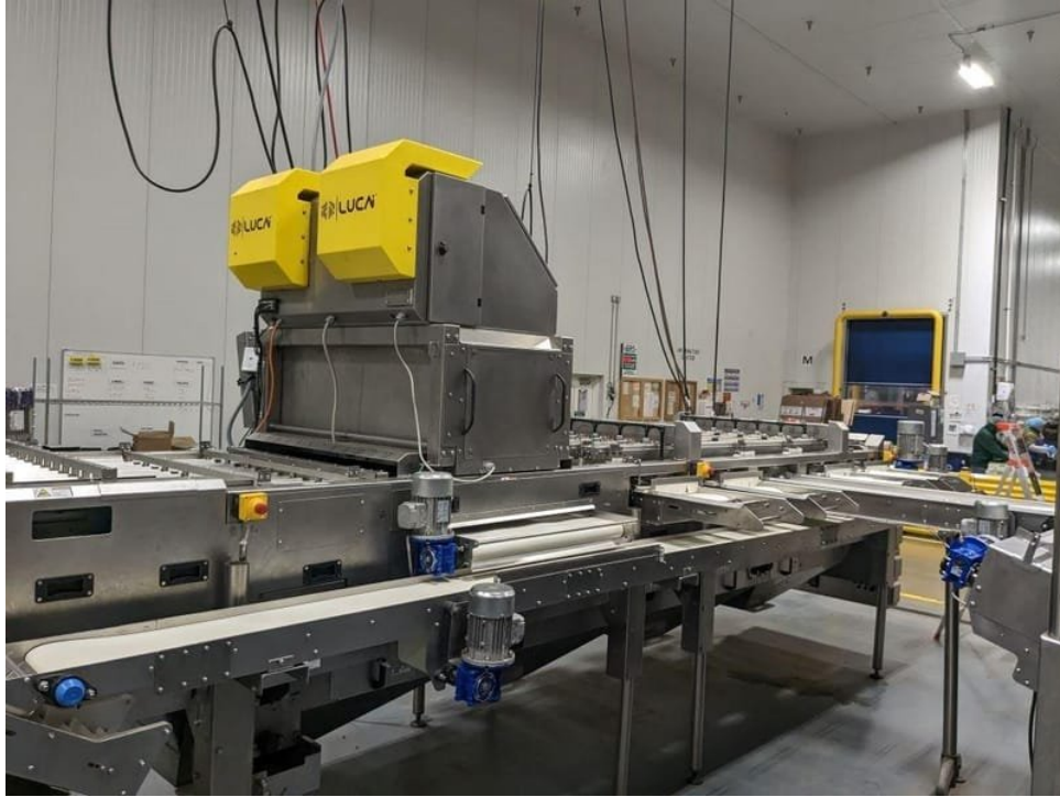
Figure 5.12: KATO260 and LUCAi™, developed by BBC Technology, a popular blueberry grading machine utilised by pack houses worldwide
