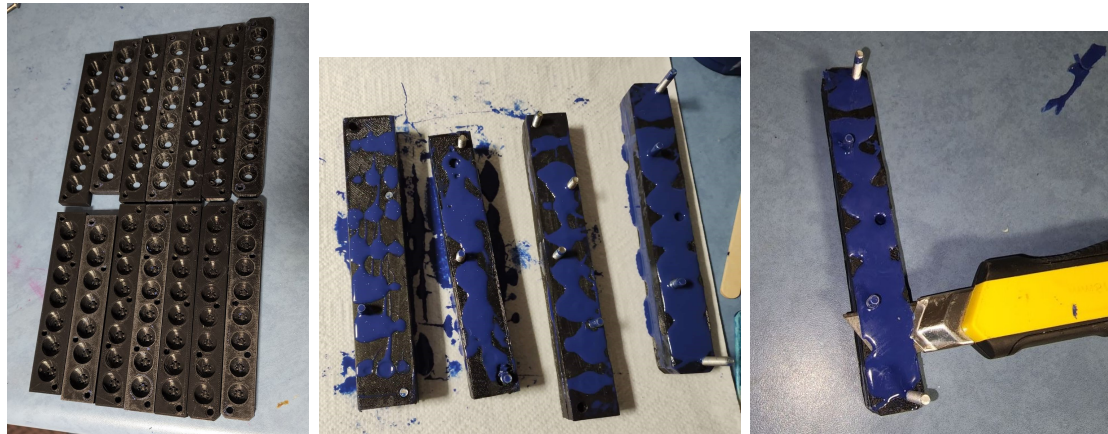
(a) 3D printed blueberry mould in various sizes (b) After pouring silicone mixtures into the moulds (c) Trim the overflow from the mould after curing
