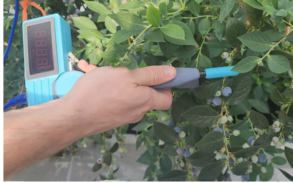
Figure 5.5: A special version of Shaker 2.0 with independent speed detection and display was created just for the trial
