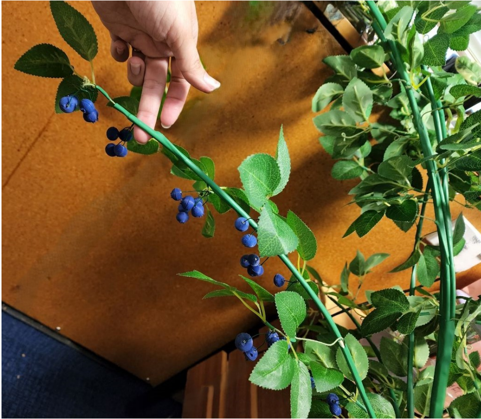
Figure 3.26: Silicone blueberries attached on the artificial cane
