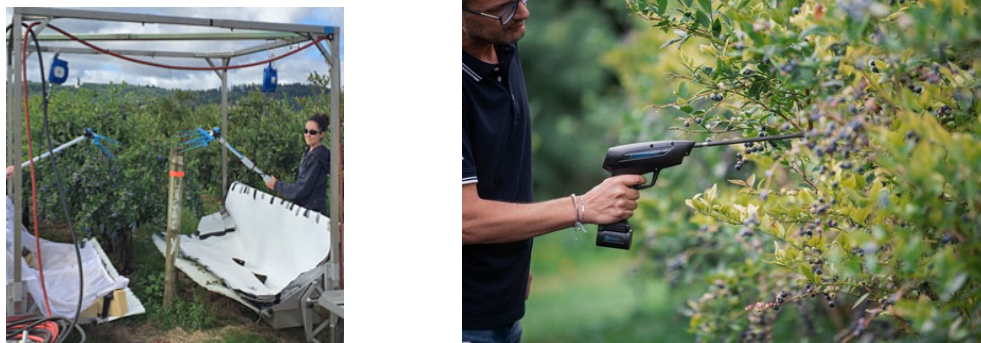
(a) Pneumatic hand-held shaker and catchment system (b) Starberry, battery-powered handheld shaker by Campagnola
