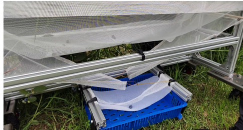
(f) Rear view shows the tray holder and third layer of netting
