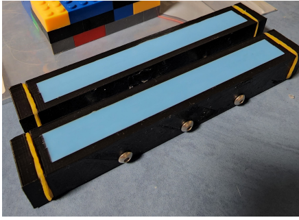
(a) 3D-printed mould for casting the silicone fingers
