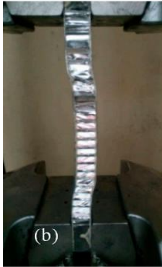
Figure 4.10: Experimental deformation pattern of honeycomb sandwich panel under axial compression showing wave-like buckling and local folding from Caiqi Zhao et al. [46]
