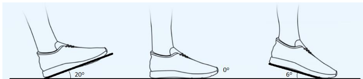
Figure 8.3. Foot-ground angles for rearfoot (left image), midfoot (centre image), and forefoot (right image) strike patterns from 2D analyses (solid lines), and anatomical landmarks used in calculating foot-ground angles.
