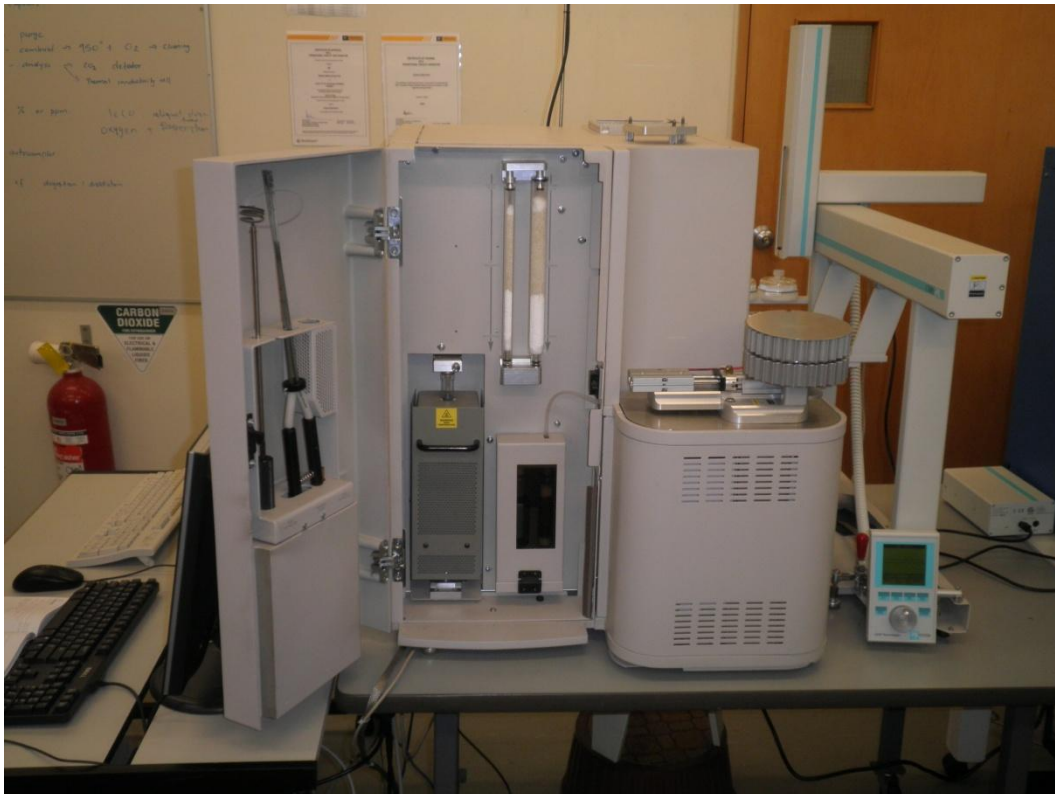
Figure 4.3: TruSpec CN Carbon/Nitrogen Determinator (LECO furnace). With two reaction columns used to purify gas from combusted sample.
