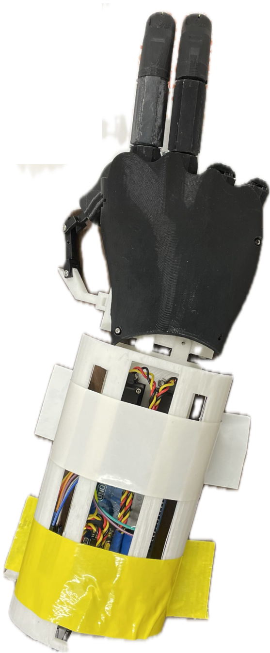
Figure 2.2. 3D printed robotic arm, only pointer and middle fingers are activated through the Myoband.
