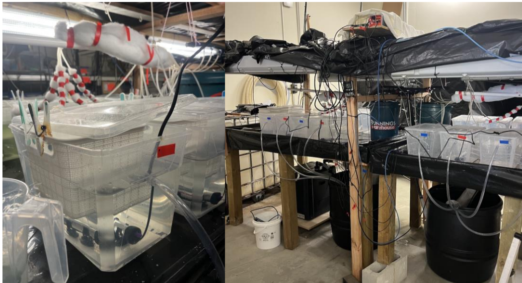
Figure 2.3. Configuration of the experimental rearing system. Individual mesh-lined baskets are suspended within the primary tanks using securing fasteners (pegs), with submersible heaters positioned at the base to ensure uniform thermal regulation across treatments.
