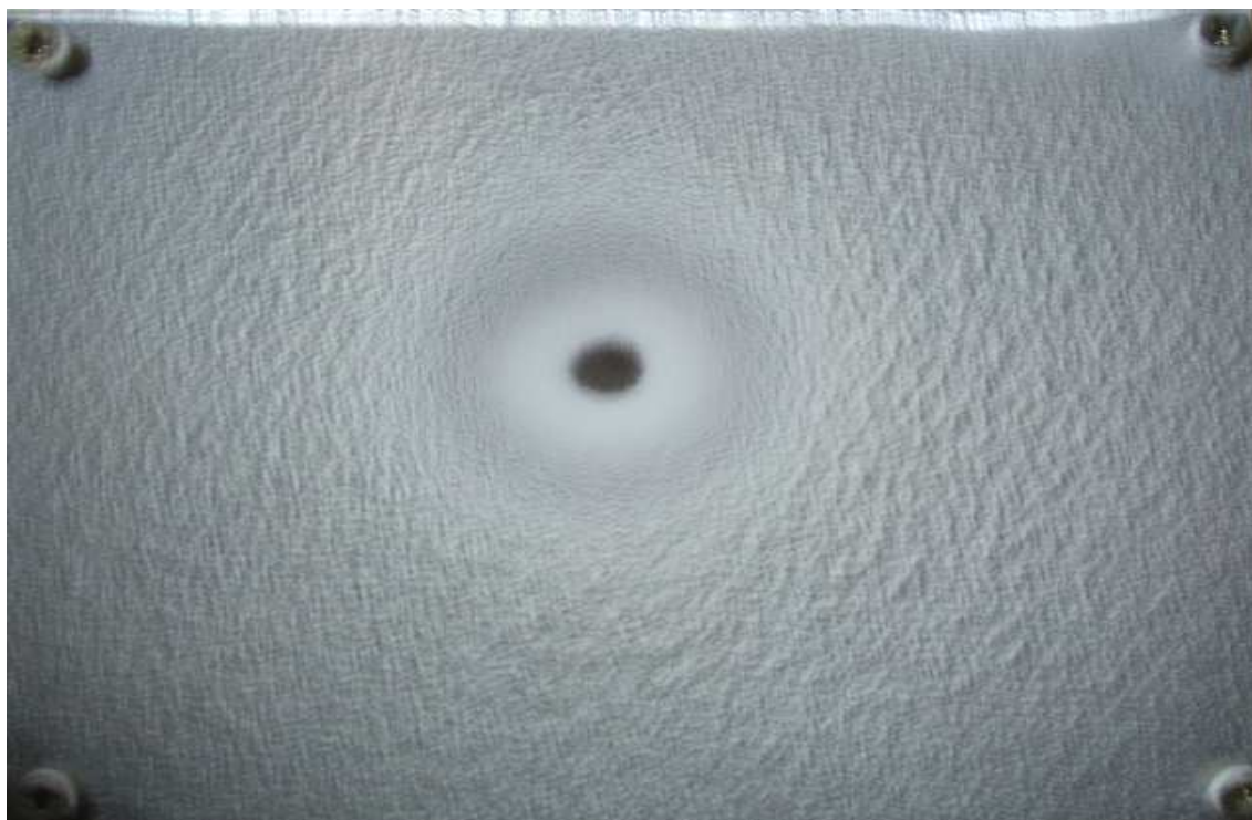
Figure A1.7 Deposit morphology at air velocity of 10.3 m/s and <45 \mu\text{m} particle fraction. T-T_g = 36.4 \text{ }^\circ\text{C} ; % Dep = 44.8 %; Centre Clear Ring Diameter = 19.4 mm.
