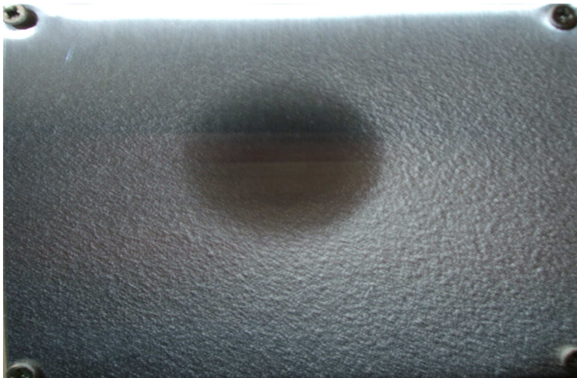
Figure A1.16 Deposit morphology at air velocity of 10.3 m/s and bulk particle fraction. T-T_g = 27.2 °C; % Dep = 8.30 %.
