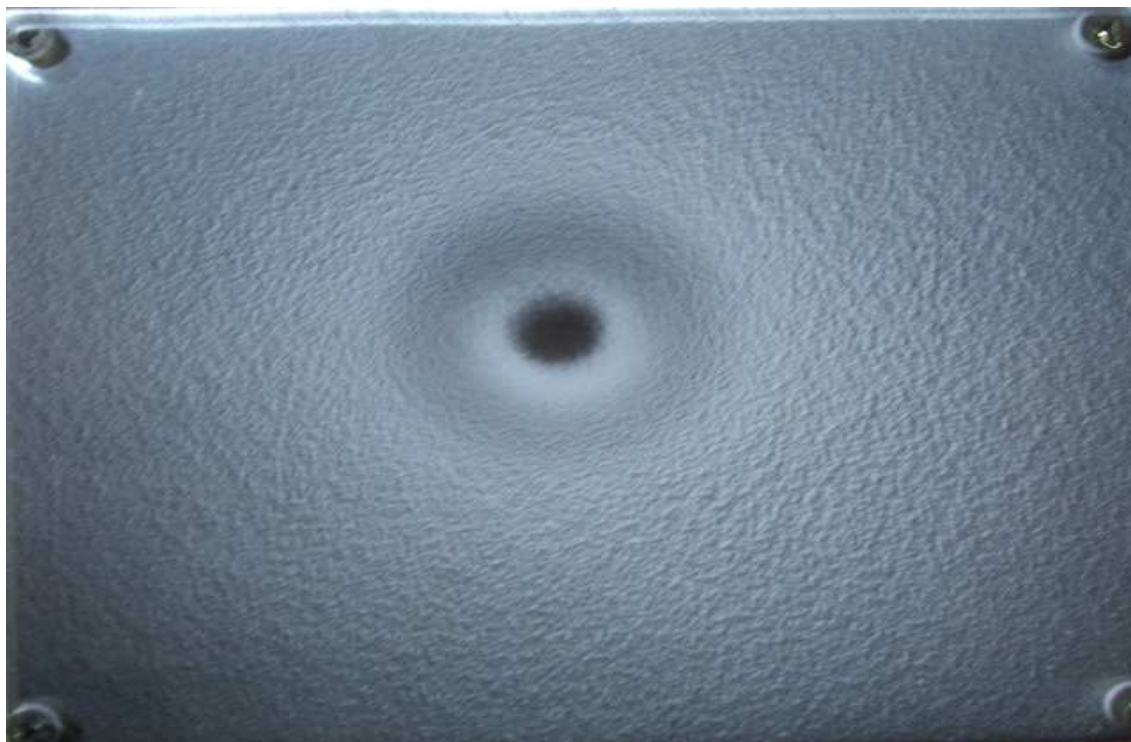
Figure A1.6 Deposit morphology at air velocity of 10.3 m/s and <45 \mu\text{m} particle fraction. T-T_g = 35.9 \text{ }^\circ\text{C} ; % Dep = 48.7 %; Centre Clear Ring Diameter = 11.5 mm.
