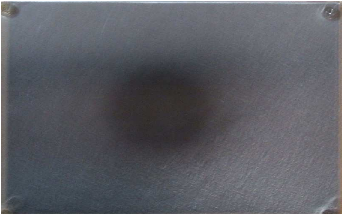
Figure A1.14 Deposit morphology at air velocity of 10.3 m/s and bulk particle fraction. T-T_g = 20.7 °C; % Dep = 3.20 %.
