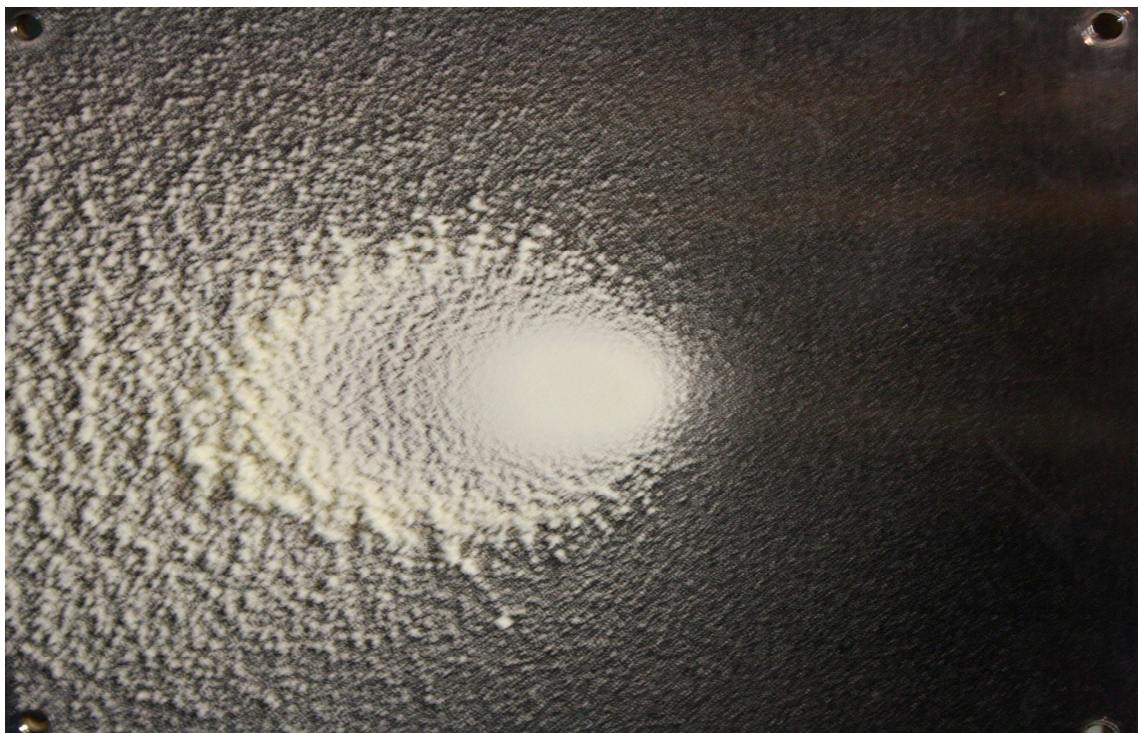
Figure A1.33 Deposit morphology at air velocity of 10.3 m/s, d_p < 45 \mu\text{m} particle size and 45^\circ of impact. T - T_g = 38.4 \text{ }^\circ\text{C} ; % Dep = 37.96 %.
