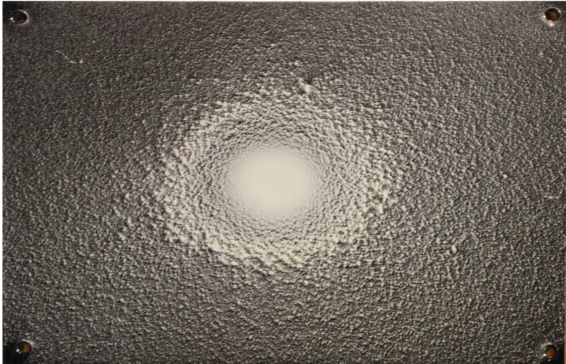
Figure A1.12 Deposit morphology at air velocity of 10.3 m/s and 45\mu\text{m} < d_p < 63\mu\text{m} particle fraction. T - T_g = 37.6\text{ }^\circ\text{C} ; % Dep = 34.12 %
