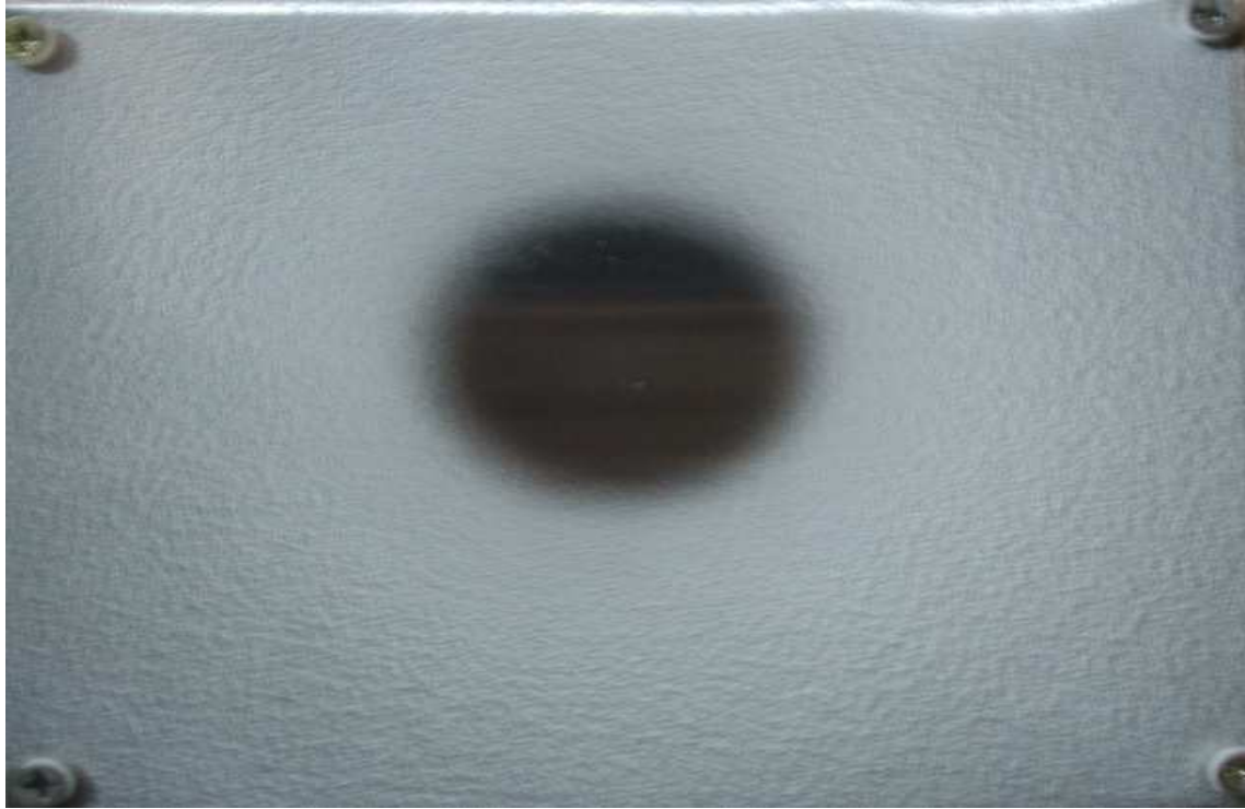
Figure A1.4 Deposit morphology at air velocity of 10.3 m/s and <45 \mu\text{m} particle fraction. T-T_g = 25.7 \text{ }^\circ\text{C} ; % Dep = 30.3 %; Centre Clear Ring Diameter = 42 mm.
