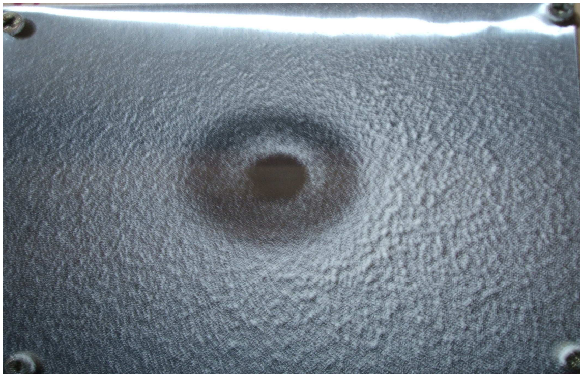
Figure A1.19 Deposit morphology at air velocity of 10.3 m/s and bulk particle fraction. T-T_g = 310.3\text{ }^\circ\text{C} ; % Dep = 23.27 %.
