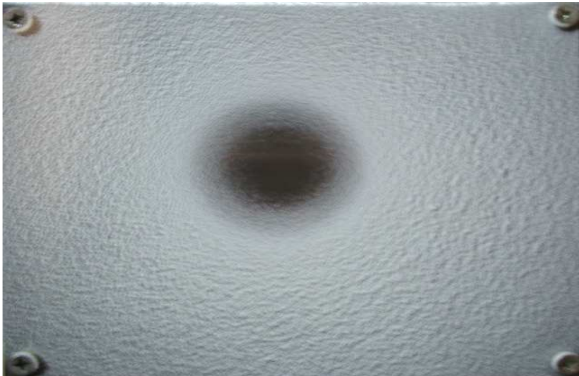
Figure A1.5 Deposit morphology at air velocity of 10.3 m/s and <45 \mu\text{m} particle fraction. T-T_g = 31.9 \text{ }^\circ\text{C} ; % Dep = 39.4 %; Centre Clear Ring Diameter = 30 mm.
