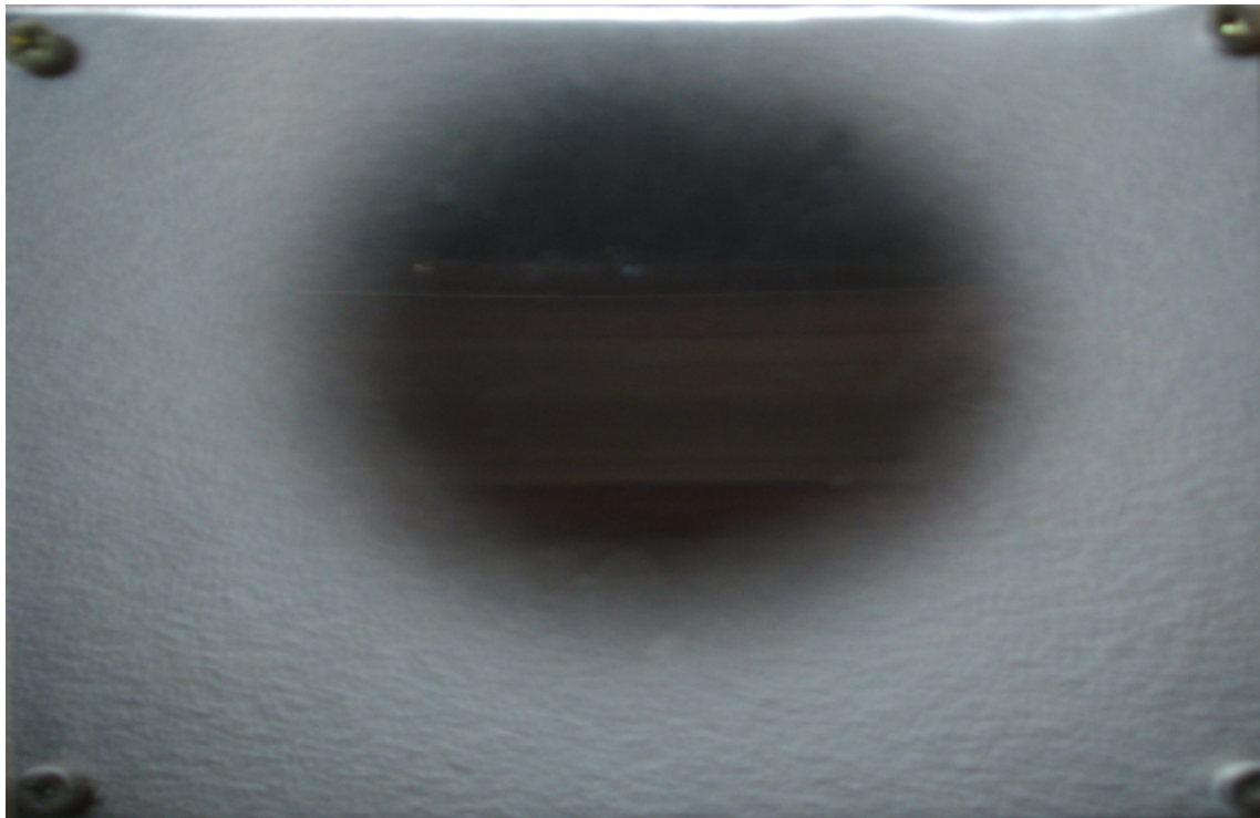
Figure A1.3 Deposit morphology at air velocity of 10.3 m/s and <45\ \mu\text{m} particle fraction. T-T_g = 19.6\ ^\circ\text{C} ; % Dep = 12.9 %; Centre Clear Ring Diameter = 68 mm.
