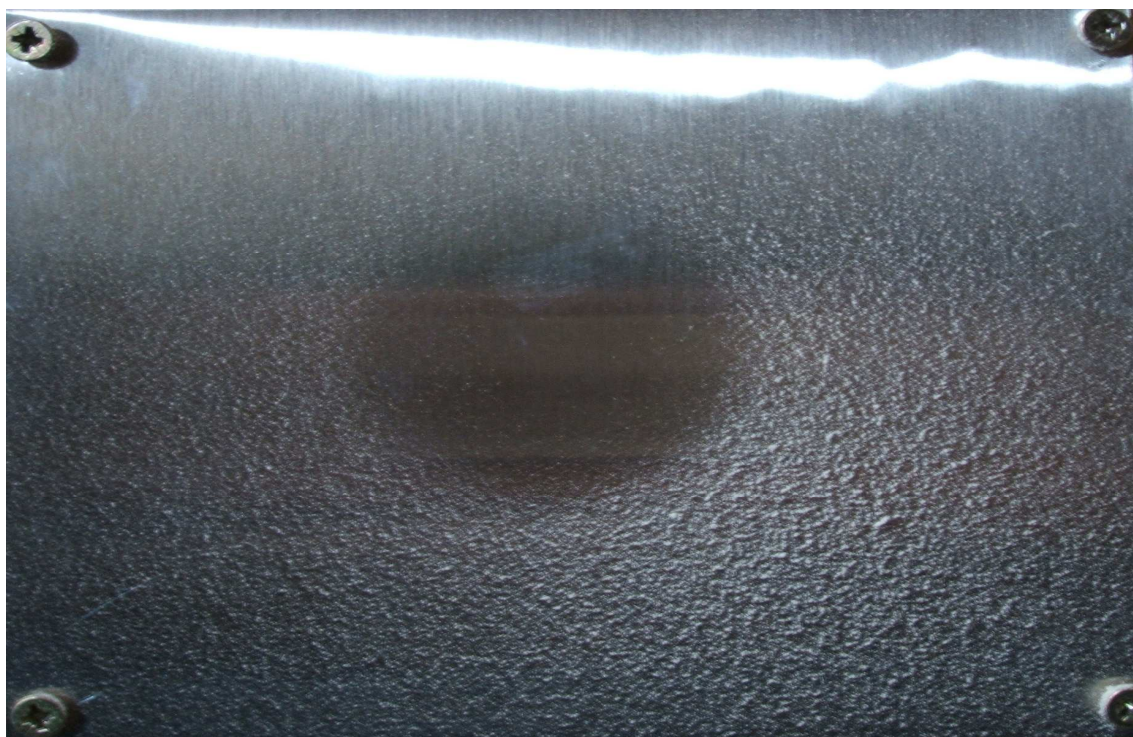
Figure A1.17 Deposit morphology at air velocity of 10.3 m/s and bulk particle fraction. T-T_g = 30.5 °C; % Dep = 13.48 %.
