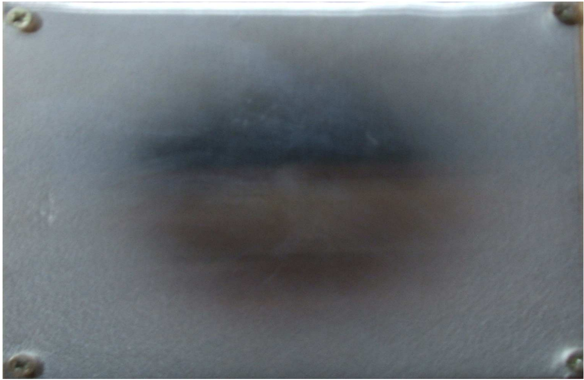
Figure A1.24 Deposit morphology at air velocity of 14.8 m/s and bulk particle fraction. T-T_g = 25.9 °C; % Dep = 1.38 %.
