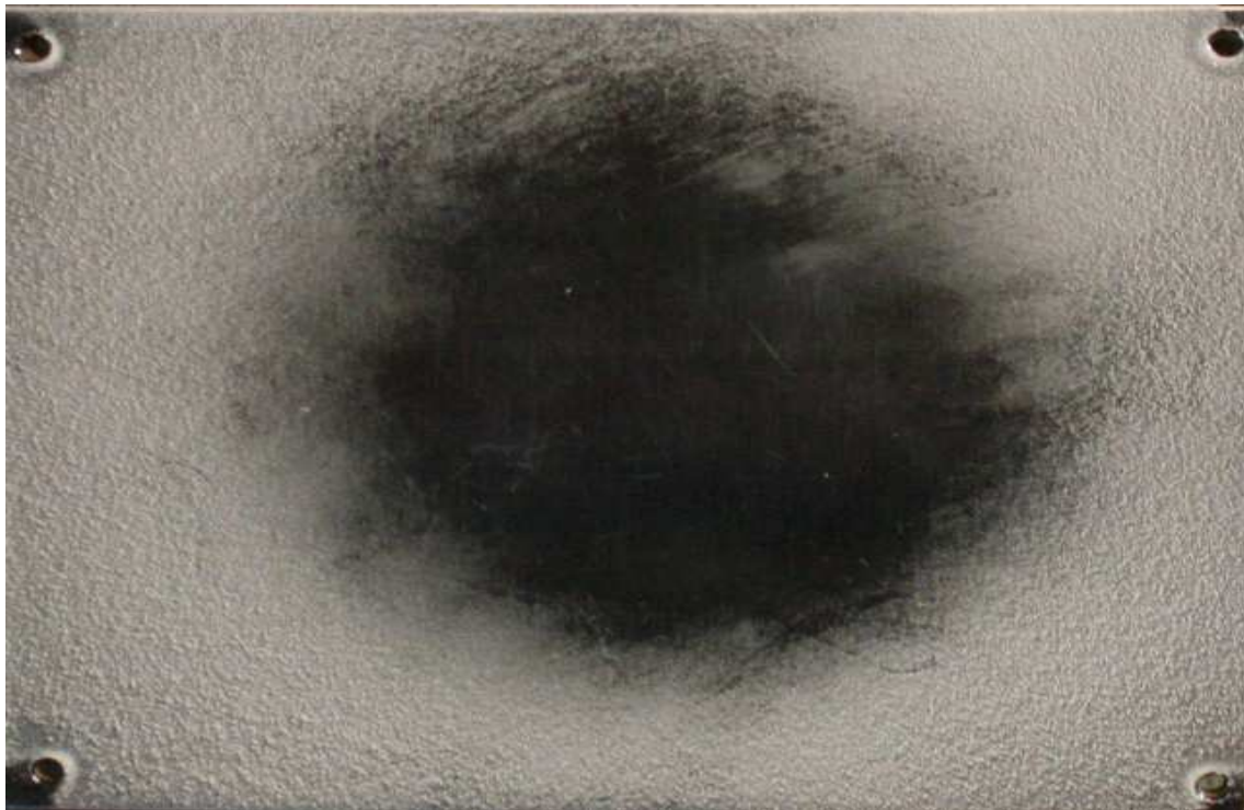
Figure A1.1 Deposit morphology at air velocity of 10.3 m/s and < 45 \mu\text{m} particle fraction. T - T_g = 15 \text{ }^\circ\text{C} ; % Dep = 8.0 %; Centre Clear Ring Diameter = 80mm.
