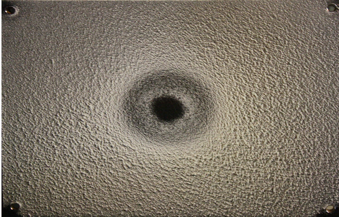
Figure A1.10 Deposit morphology at air velocity of 10.3 m/s and 45\mu\text{m} < d_p < 63\mu\text{m} particle fraction. T - T_g = 28.8\text{ }^\circ\text{C} ; % Dep = 28.98 %.
