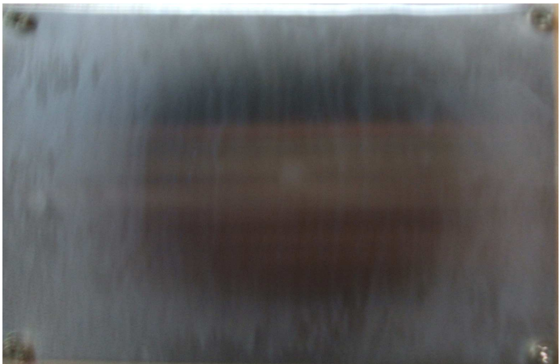
Figure A1.23 Deposit morphology at air velocity of 14.8 m/s and bulk particle fraction. T-T_g = 21.4 °C; % Dep = 0.4 %.
