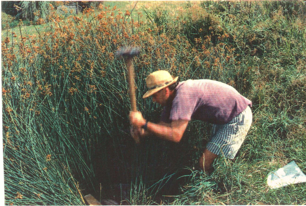
Plate 8. The hard work of driving large corers (18 per wetland) into the gravel substratum to extract roots and rhizomes - Final sampling, January 1992.
