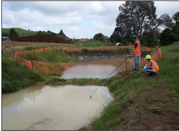
Fig. 4.5: Sample collection using a battery-driven pump (Photo courtesy of L. Ward, 2006).
