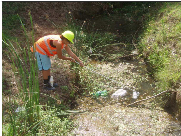
Fig. 4.6: Sample collection using the “bucket-on-a-pole” (Photo courtesy of E. McElhannan, 2007).
