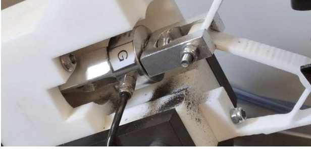
Figure 9: Filings that fell onto the gripper mounting block because of abrasion of the aluminum connector parts.
