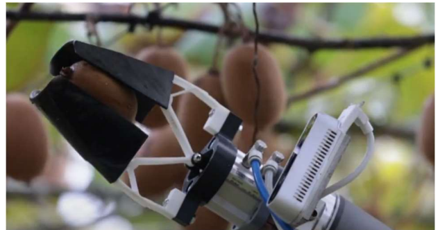
Figure 1: A compliant mechanism robotic gripper-end effector device equipped on a UR5e harvesting kiwifruit in the field [10].
