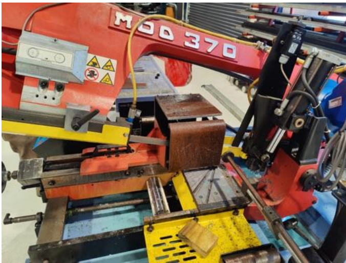
Figure 16: (a) Vertical saw cutter machine and (b) 400-grade rectangular section specimen location
