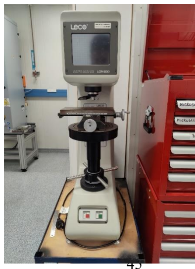
Figure 21: LCR 500- Used for both Rockwell and Brinell hardness test
