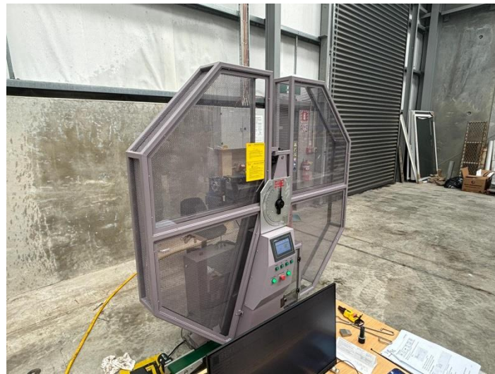
Figure 25: Illustration of Charpy impact test available in the lab.
