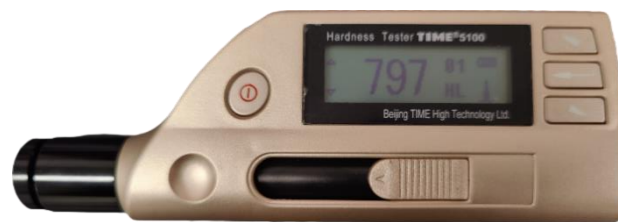
Figure 3: Depiction of the Leeb hardness tester.
