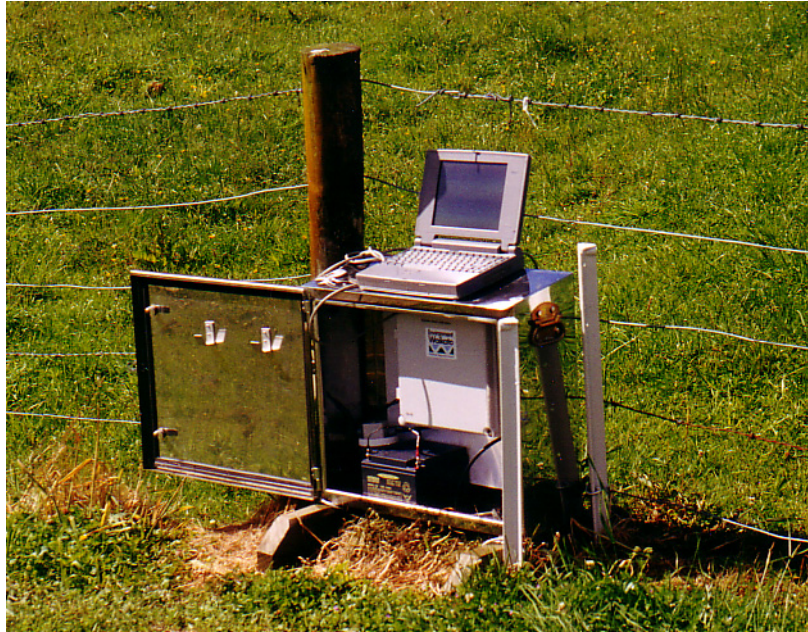
Fig. 2.2. Automatic level recorder on the Matarawa Stream inlet.
