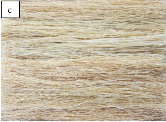
Fig.1.Harakeke macrographs showing (a) harakeke plant, (b) harakeke fibre bundles and (c) aligned harakeke fibre mat
