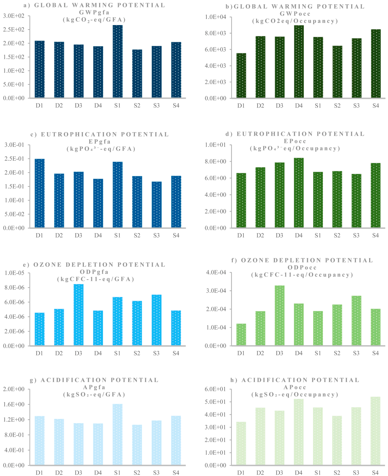
Fig. 3. Environmental Impacts per gross floor area (GFA) and per occupancy for each building.
