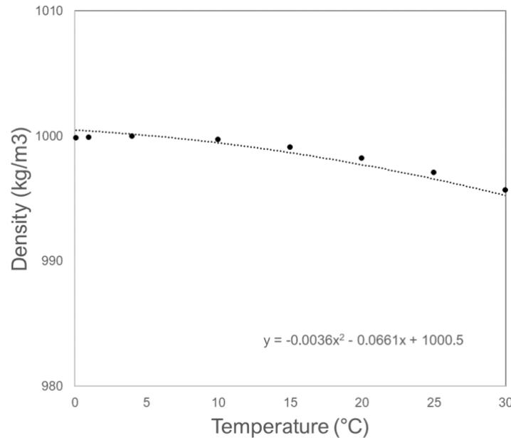
Figure 2-4: Water Density-Temperature Correlation (Engineering Toolbox, 2022)
