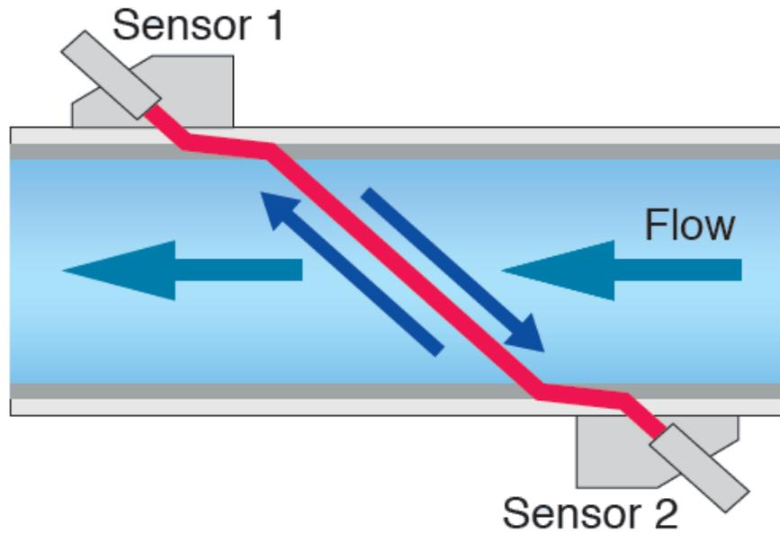
Figure 4-4: Example of a Transit Time Ultrasonic Flow Meter Layout (Fuji Electric, 2022)
