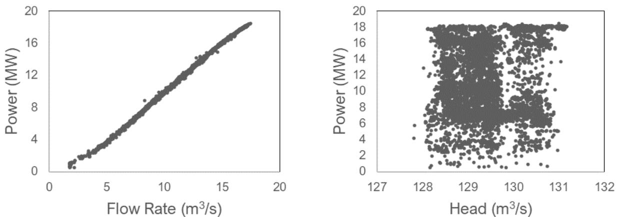
Figure 5-2: Predictor Variable Relationship, Unit 6 Flow Rate-Power (Left), Head-Power (Right)
