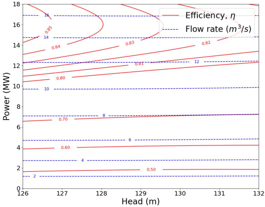
Figure 10-17: Hill Diagram Unit 7
