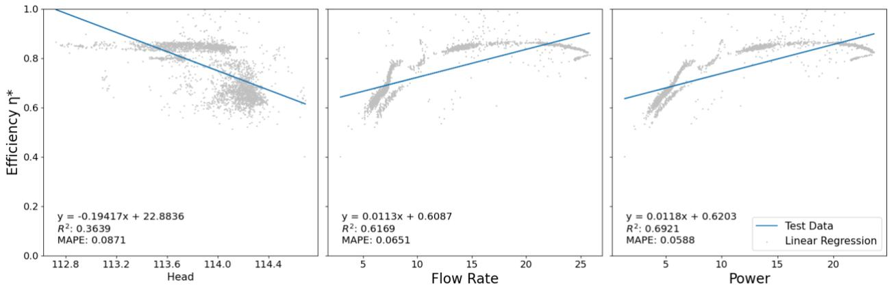
Figure 10-10: Unit 4 Only Linear Regression Plots Against Validation Data
