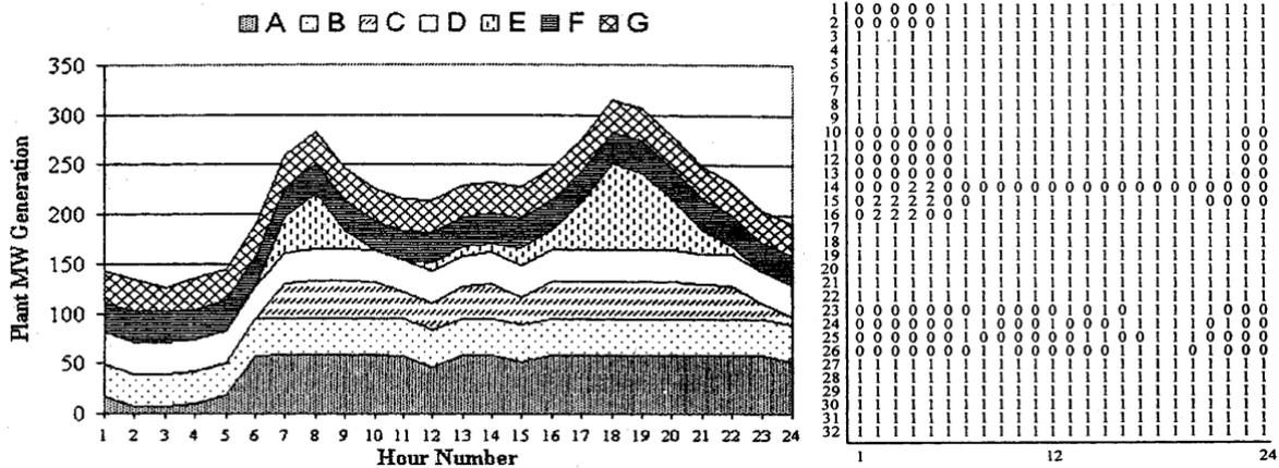
Figure 2-8: Scheduling (Left) and Hourly Hydro Unit Commitment Status (Right) for System 2 (Chang et al., 2001).
