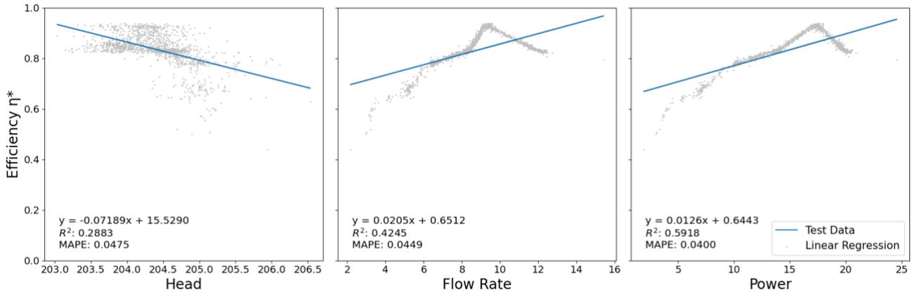
Figure 10-9: Unit 3 Linear Regression Plots Against Validation Data
