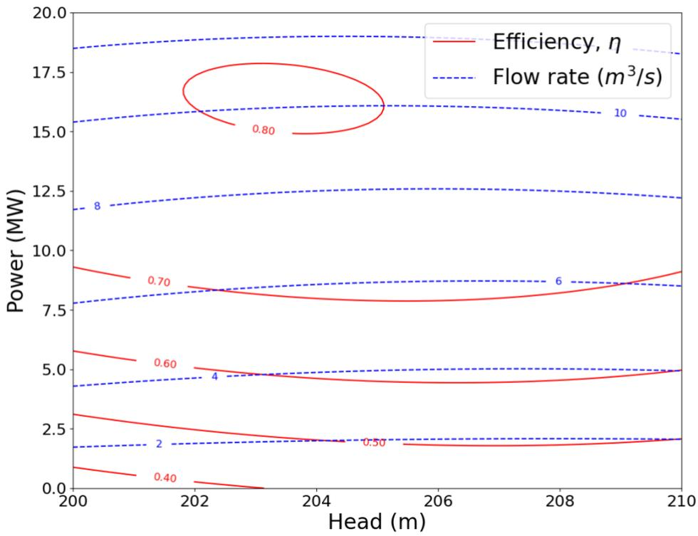
Figure 10-19: Hill Diagram Unit 2
