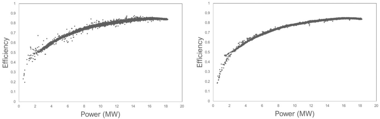
Figure 4-2: Power-Efficiency Plots, Instant Data (Left) & Averaged Data (Right) at 1 Minute Interval
