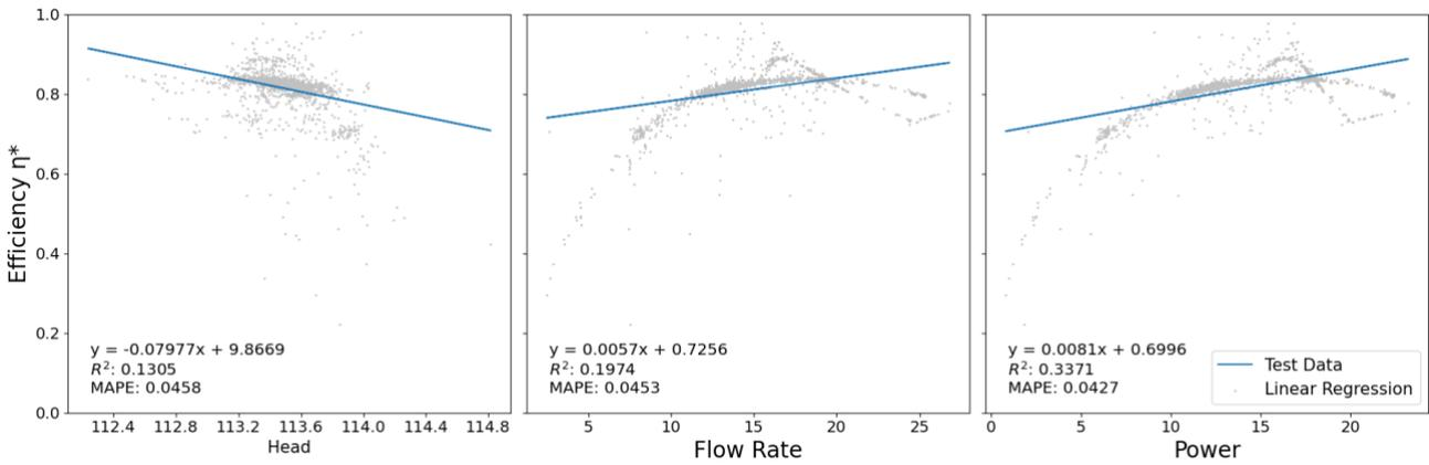
Figure 10-13: Unit 5 Tandem Linear Regression Plots Against Validation Data
