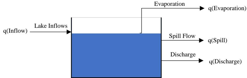
Figure 6-1: Mass Balance for a Standard Hydropower Reservoir
