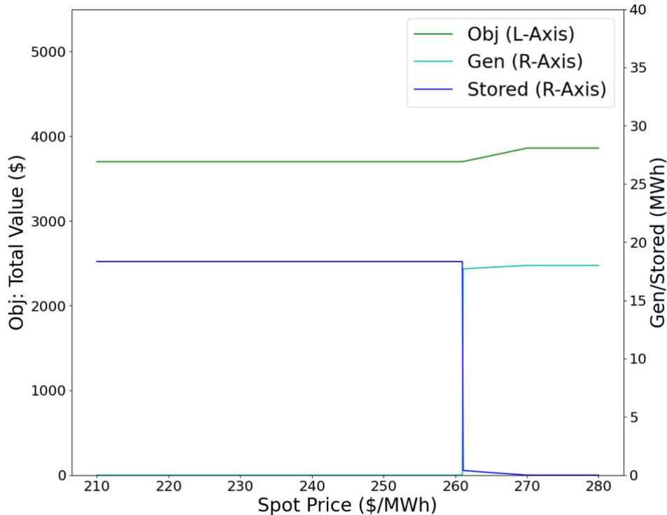
Figure 7-2: Generation-Stored-Startup Value Optimisation with Increasing Spot Price
