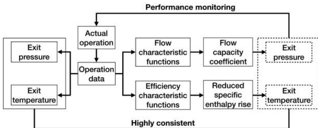
Figure 2-3: J. Yu et al.(2020)'s Digital Twin schematic diagram
