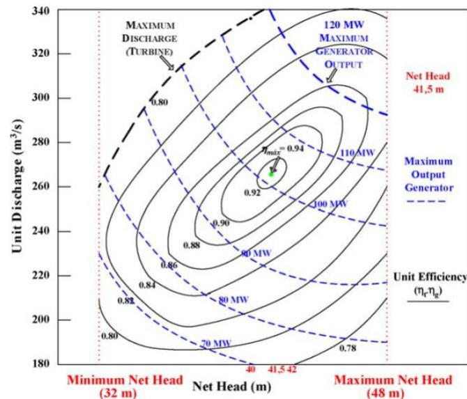
Figure 2-5: Example of a Turbine Hill Diagram (Finardi & da Silva, 2005)
