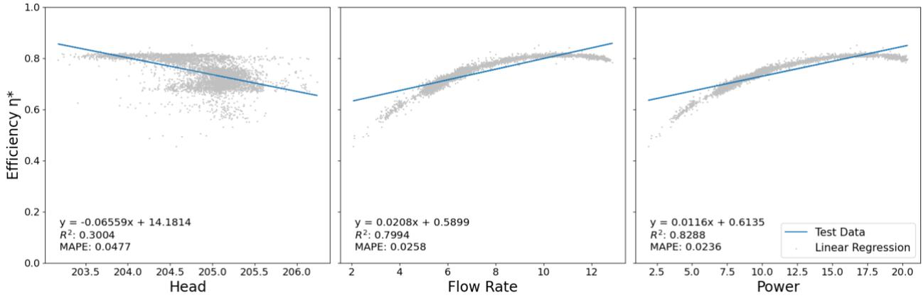
Figure 10-7: Unit 1 Linear Regression Plots Against Validation Data
