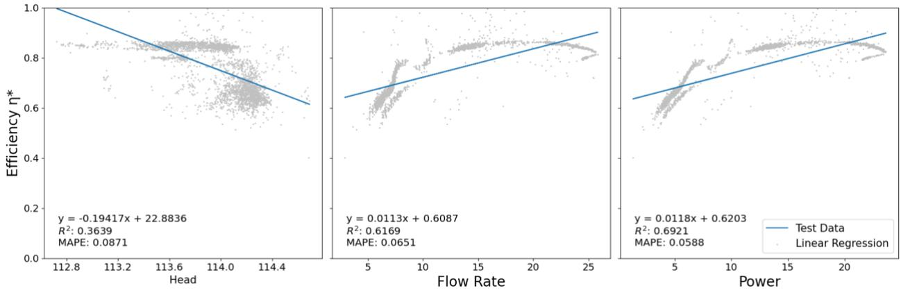
Figure 10-12: Unit 5 Only Linear Regression Plots Against Validation Data
