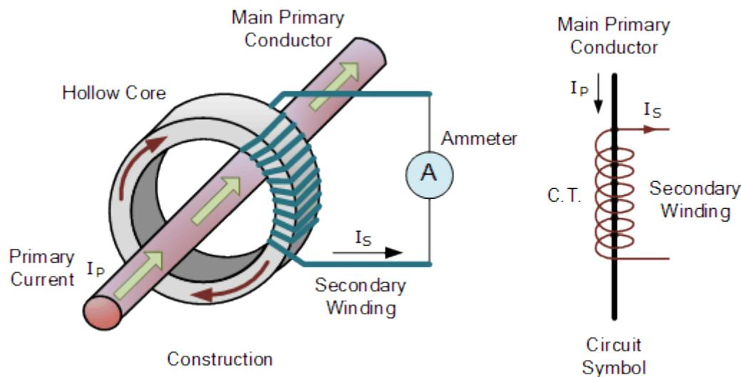
Figure 4-5: Components of a Current Transformer (Electronics Tutorials, 2022)
