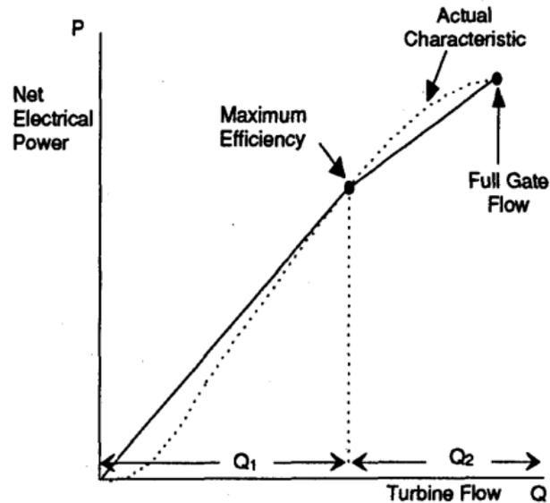
Figure 2-6: Unit Characteristic Performance Curve and Piecewise Characteristic by Piekutowski and Liwinowicz (1994)
