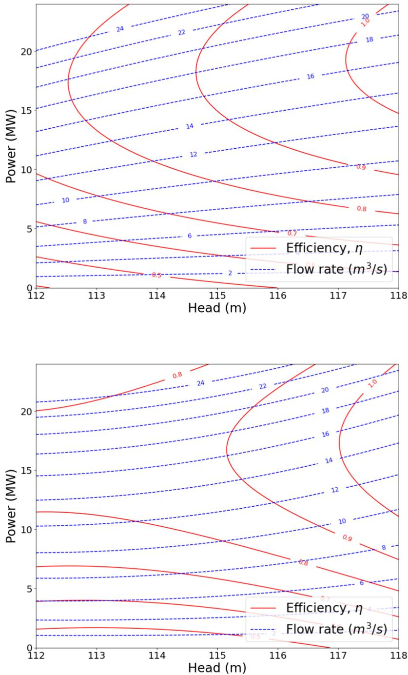
Figure 5-4: Hills diagrams for Unit 4 (Top) and Unit 5 (Bottom)
