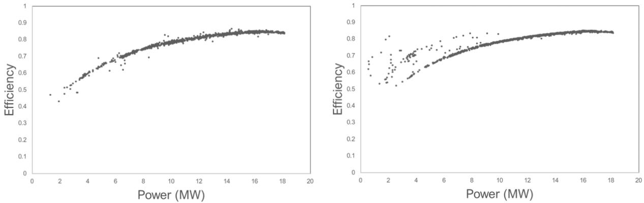
Figure 4-1: Power-Efficiency Plots, Instant Data (Left) & Averaged Data (Right) at 1 Hour Interval
