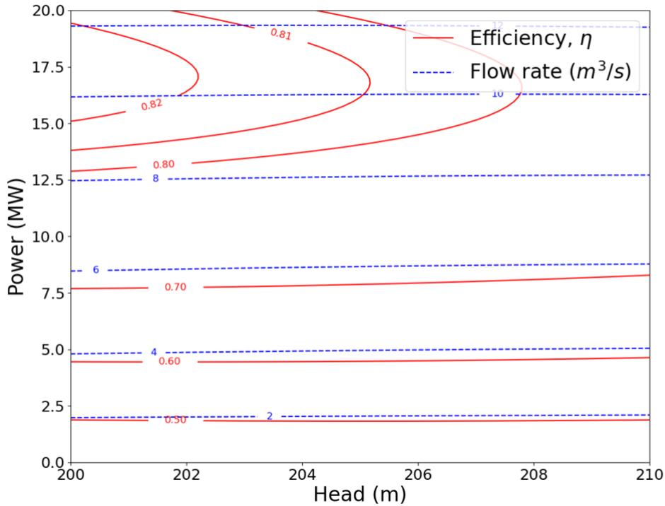
Figure 10-18: Hill Diagram Unit 1
