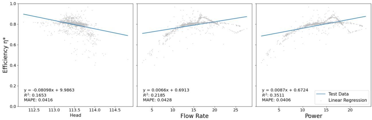
Figure 10-11: Unit 4 Tandem Linear Regression Plots Against Validation Data
