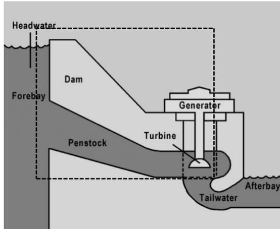
Figure 6-2: Hydro Dam with Energy Balance Boundary (U. S. Department of the Interior: Bureau of Reclamation, 2005)
