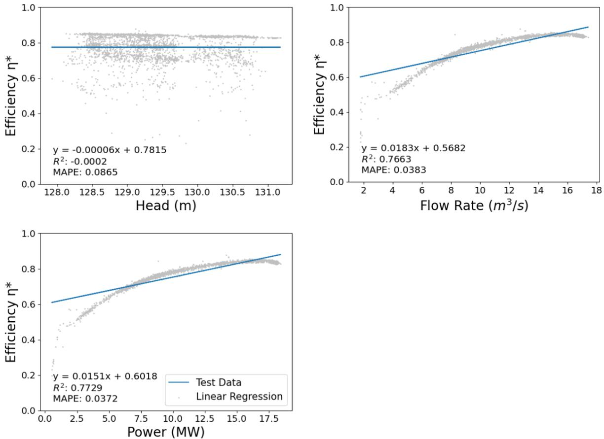
Figure 5-1: Unit 6 Linear Regression Plots Against Validation Data
