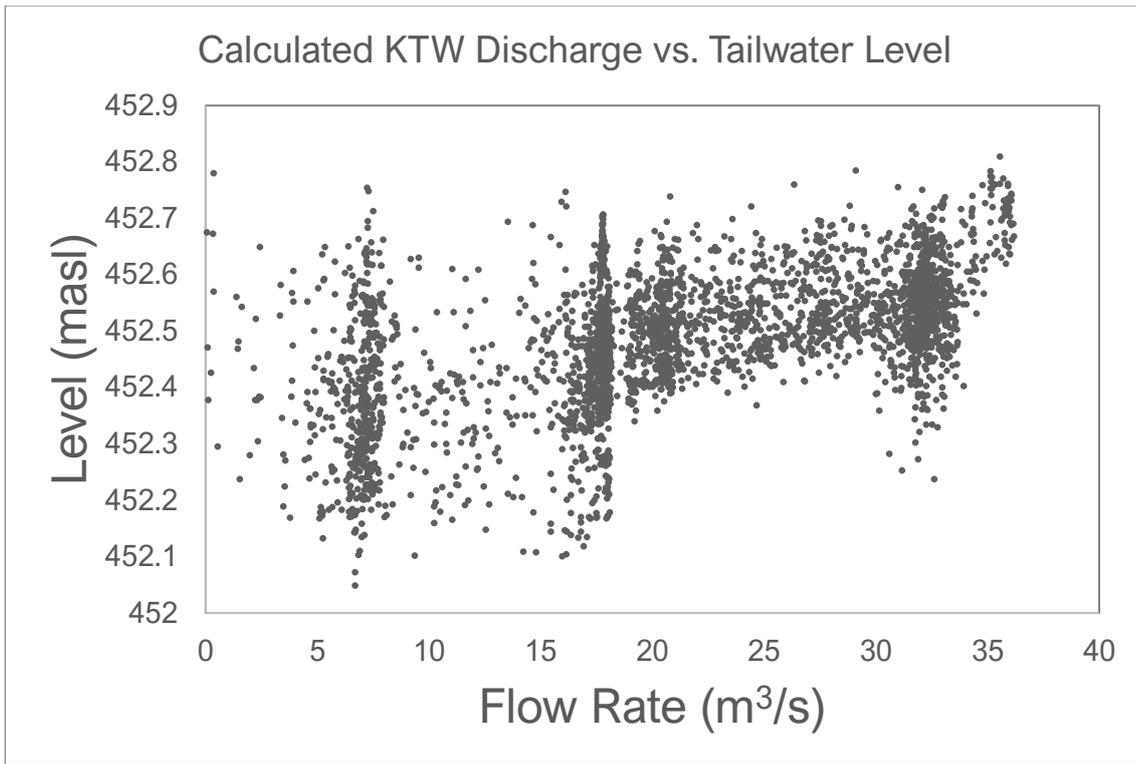
Figure 10-15: L1 Tailwater Variation from Flow
