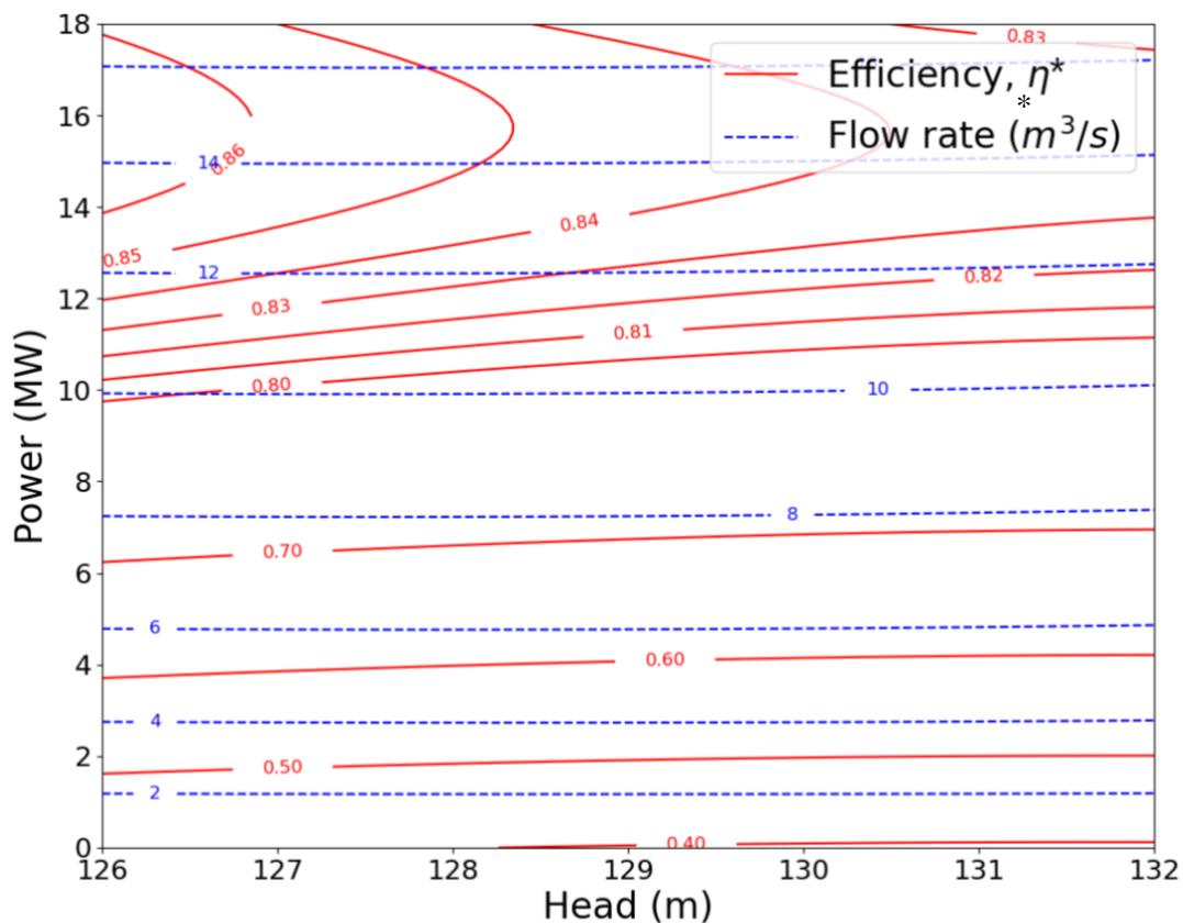
Figure 5-3: Hill diagram for Unit 6
