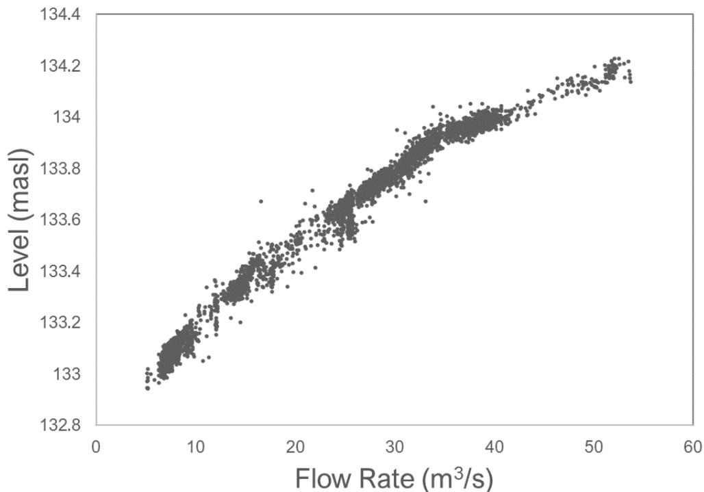
Figure 6-5: Piripaua Tailwater Head Variation, Flow Dependence
