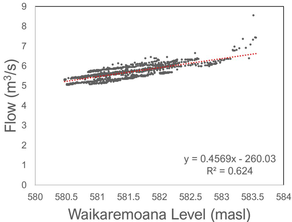
Figure 3-5: Waikaremoana Leakage Flow and Lake Level Relationship
