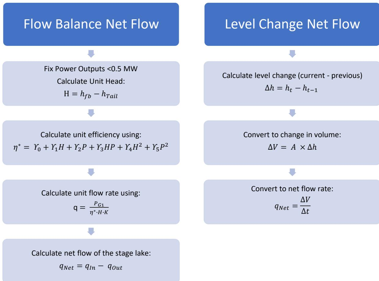
Figure 6-7: Calculation Process for Flow Balance and Level Reconciliation
