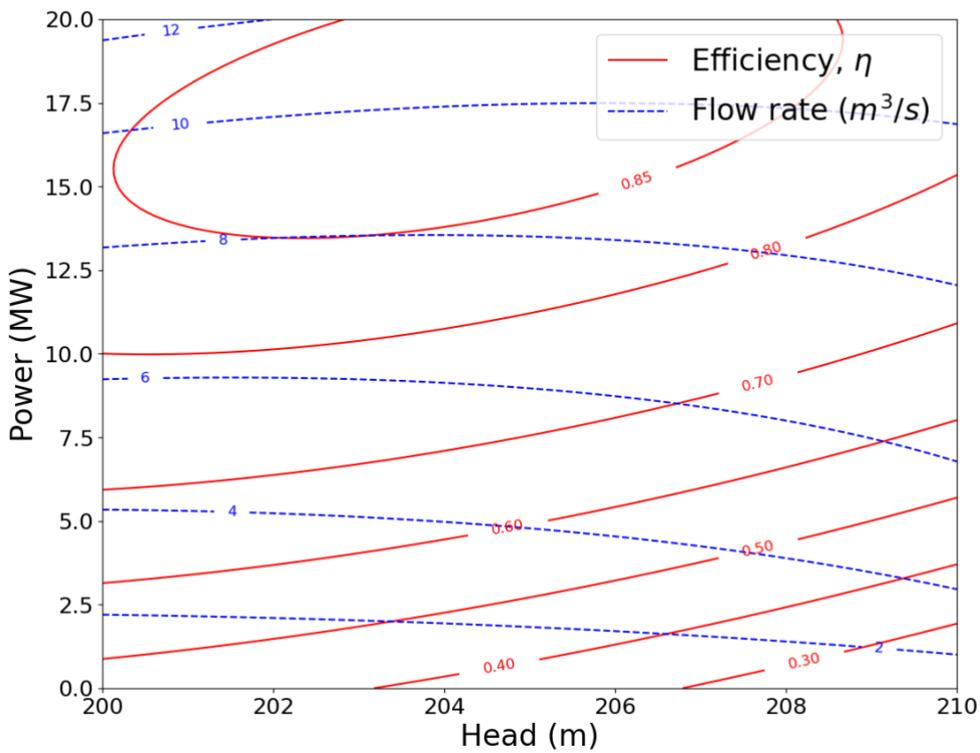
Figure 10-20: Hill Diagram Unit 3
