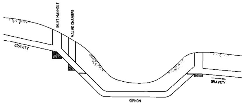
Figure 10-4: Example Diagram of an Inverted Water Siphon (Miles, 2009)
