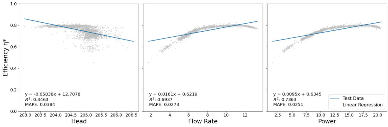
Figure 10-8: Unit 2 Linear Regression Plots Against Validation Data
