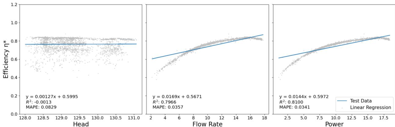
Figure 10-6: Unit 7 Linear Regression Plots Against Validation Data
