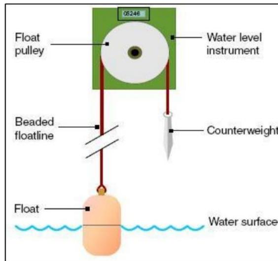
Figure 4-3: Shaft Encoder Type Level Transducer (Taylor, 2019)
