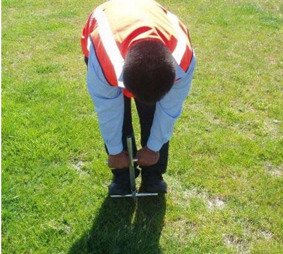
Figure 7.2: Soil core cutter.
