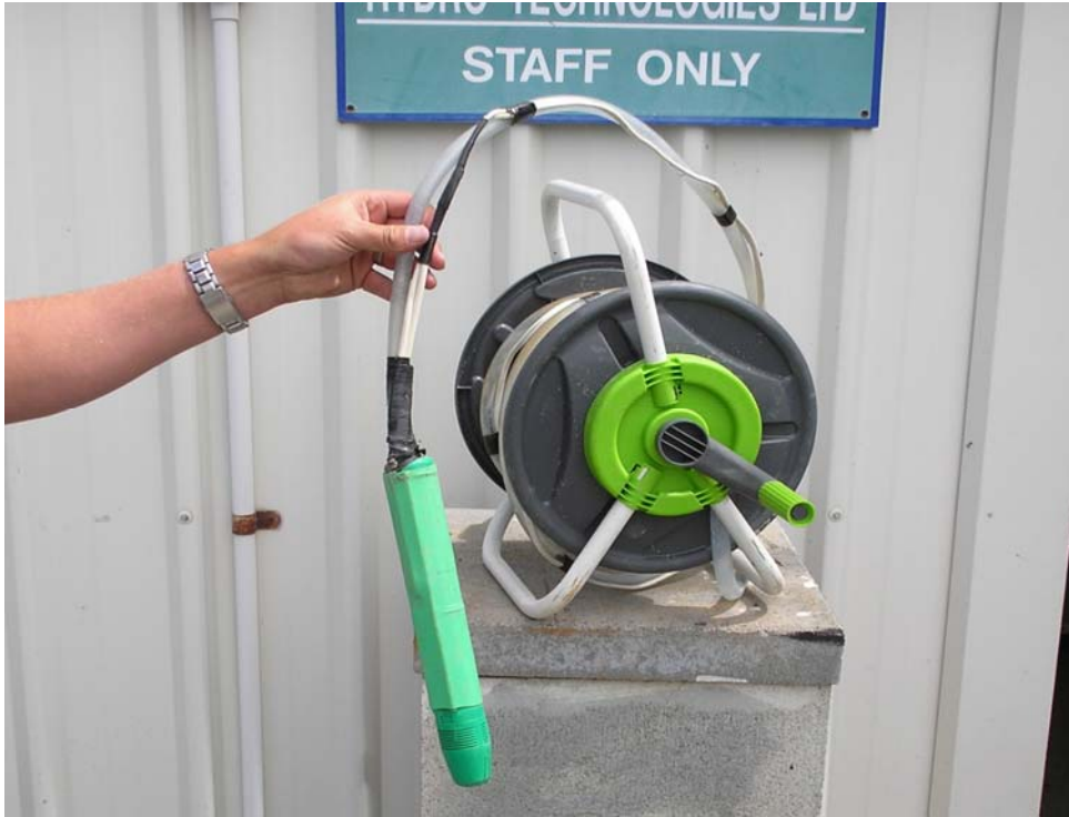
Figure 4.1: One of the pumps used to collect bore samples.
