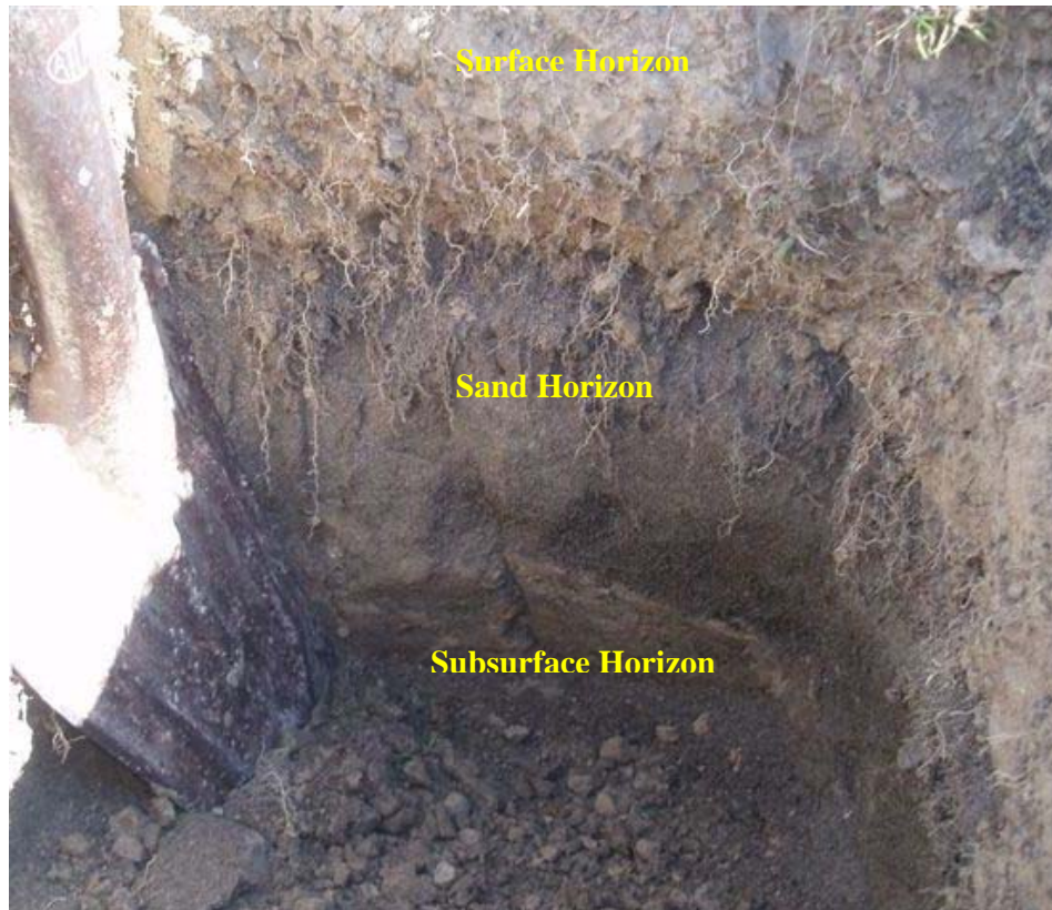
Figure 7.3: Subsurface horizon sample collection in the landfill cap.
