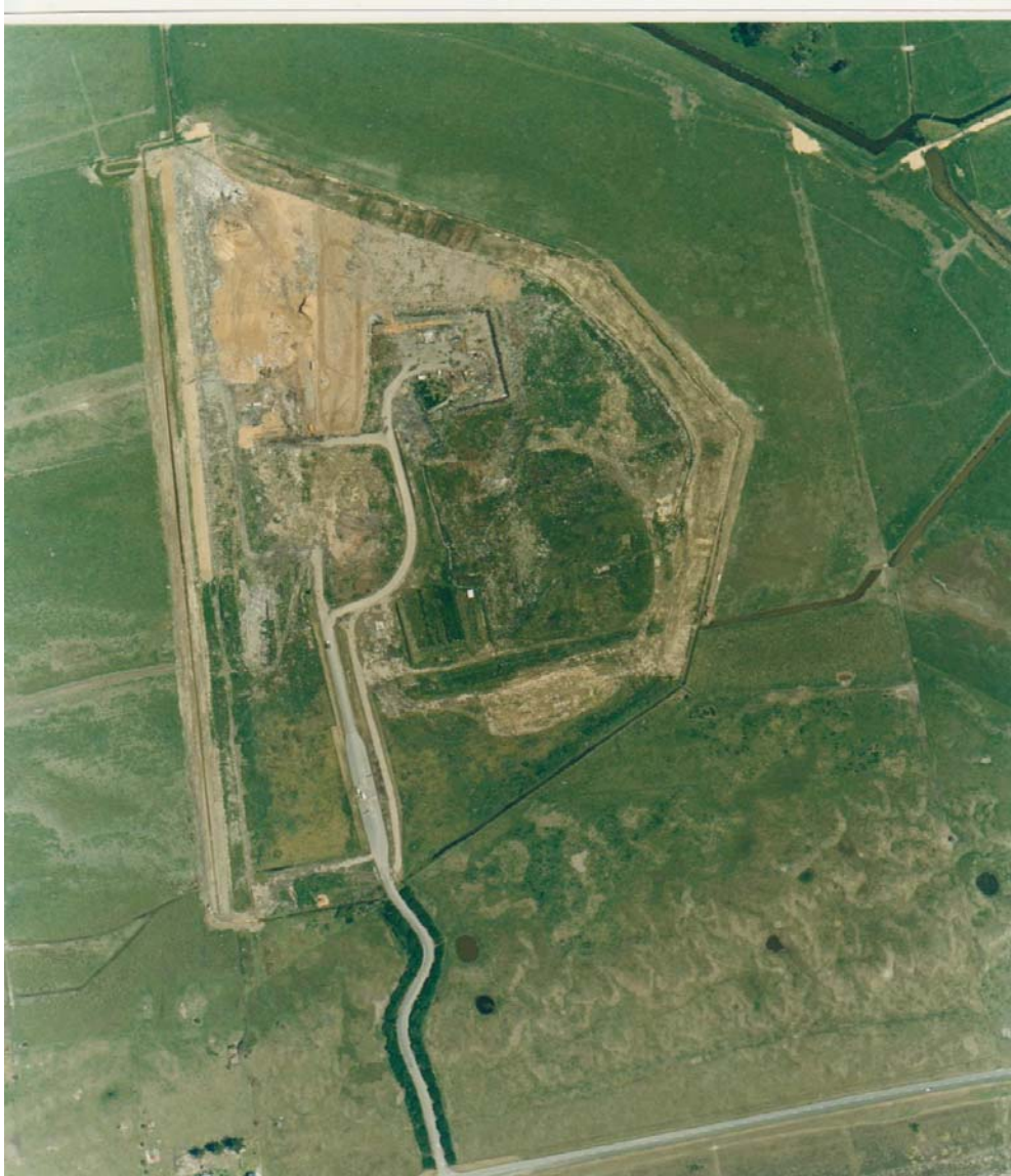
Figure 3.1: Paokahu Landfill December 2000, showing the active tip face in the northern corner.
