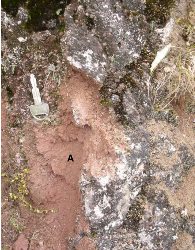
Figure 4.10 – Altered andesite outcrop exhibiting a readily disaggregated nature. The nature of this lithotechnical unit is evidence of its weak field strength. Weathered surfaces of the altered andesite appear grey, while freshly exposed surfaces appear reddish (as indicated by ‘A’). Photo taken at site 40. Key for scale.
