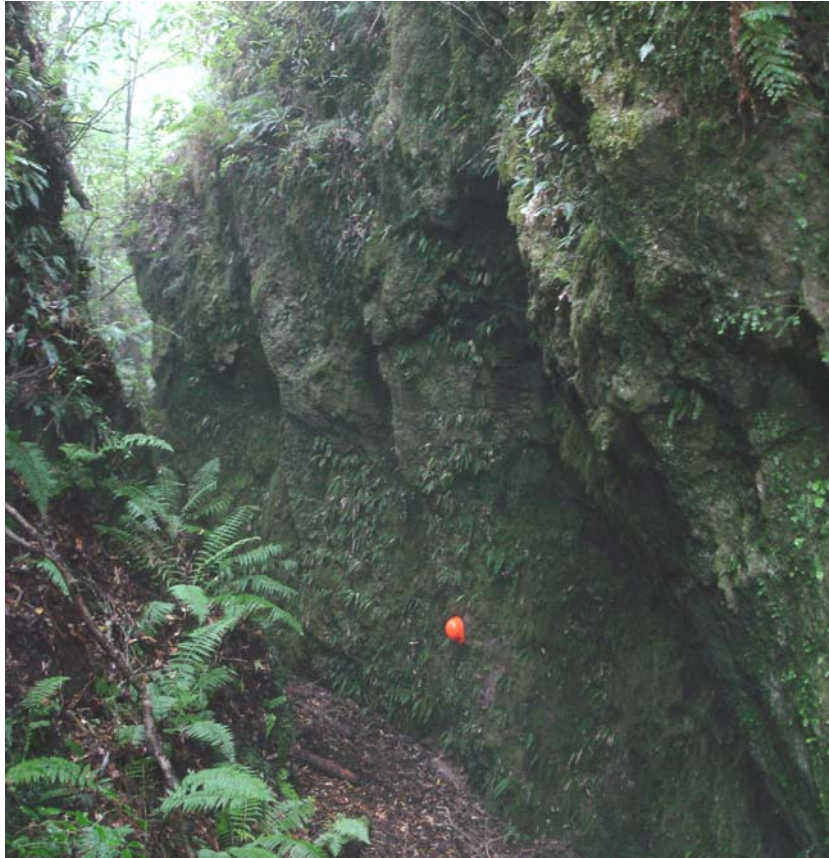
Figure 4.8 – Discontinuity sets in the scoriaceous andesite. Major discontinuity sets are very apparent; however, the sub-canopy location and associated blankets of moss-like vegetation mean a clean view of minor discontinuities is difficult. Note the canyon-like location of the outcrop. Photo taken at site 33. Safety helmet for scale.
