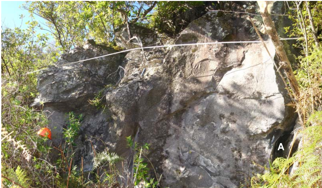
Figure 4.12 – Indurated dacite outcrop exhibiting very wide discontinuity apertures (as shown by ‘A’ in the lower right of the above figure). Photo taken at site 52. Safety helmet for scale.
