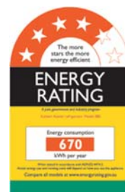
Figure 1: An Energy Rating Label which gives an indication on the appliances energy usage and energy efficiency. Image from [6]
