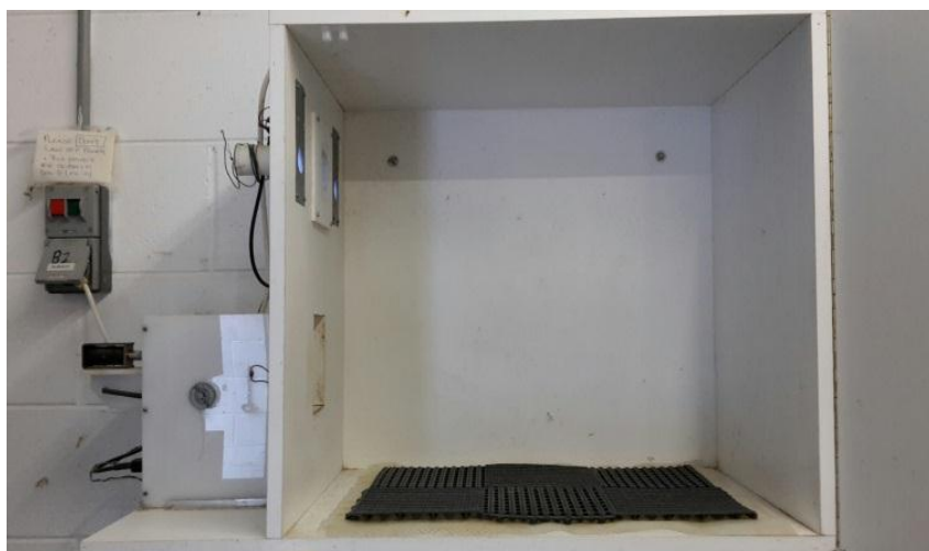
Figure 1.1. Side view of operant task chamber and external food magazine on bottom left.
