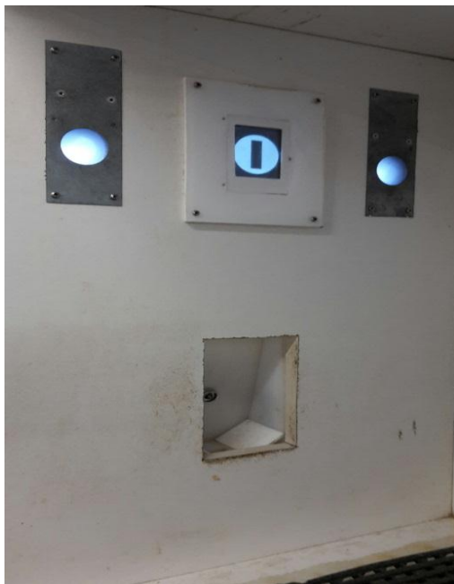
Figure 1.3. Operant chamber screen (centre), showing vertical rectangle (positive cue) presentation, response manipulanda to left and right of screen and food access opening below the screen, on short wall.
