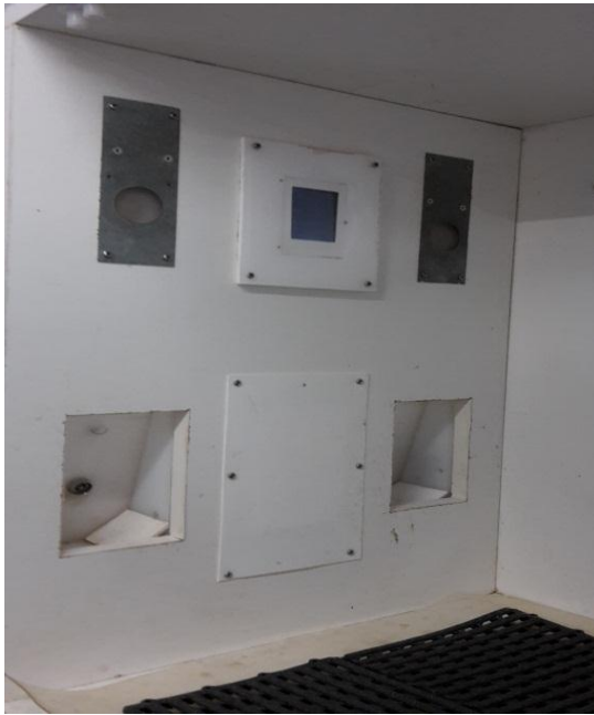
Figure 1.7. Modified chamber with access to two food magazines
