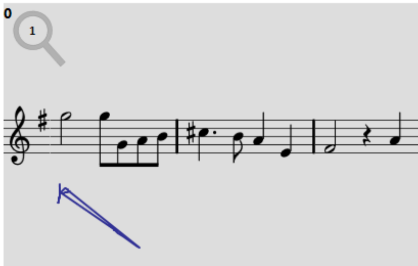
Figure 81 Phantom touch detected when hand gets close to the screen. A users' attempt at 'Text and Dynamics' annotation at zoom level 1 (actual size).
