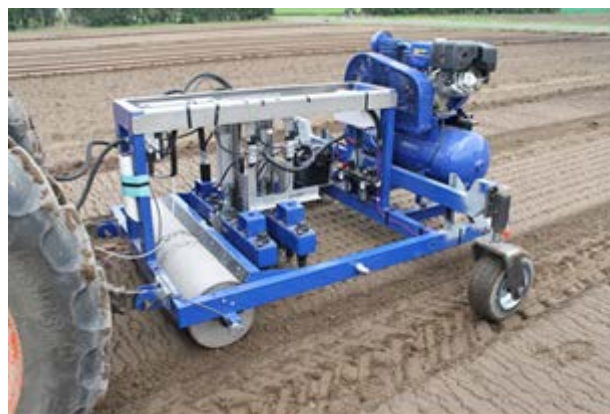
Fig. 5 – Completed mechatronic dibbling machine during testing
