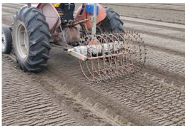
Fig. 2 – Radiata Pine dibbling machine
