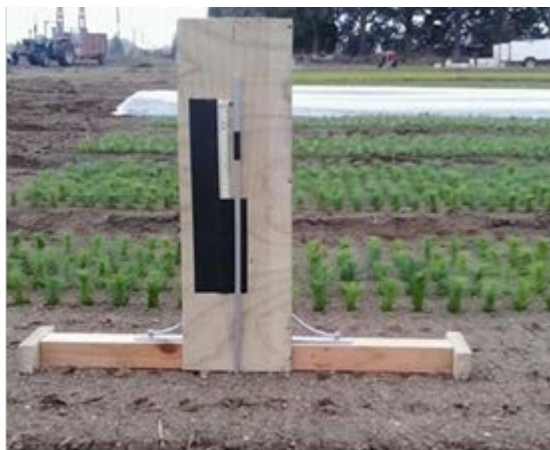
Fig. 6 – Measuring device for hole depth and angle
