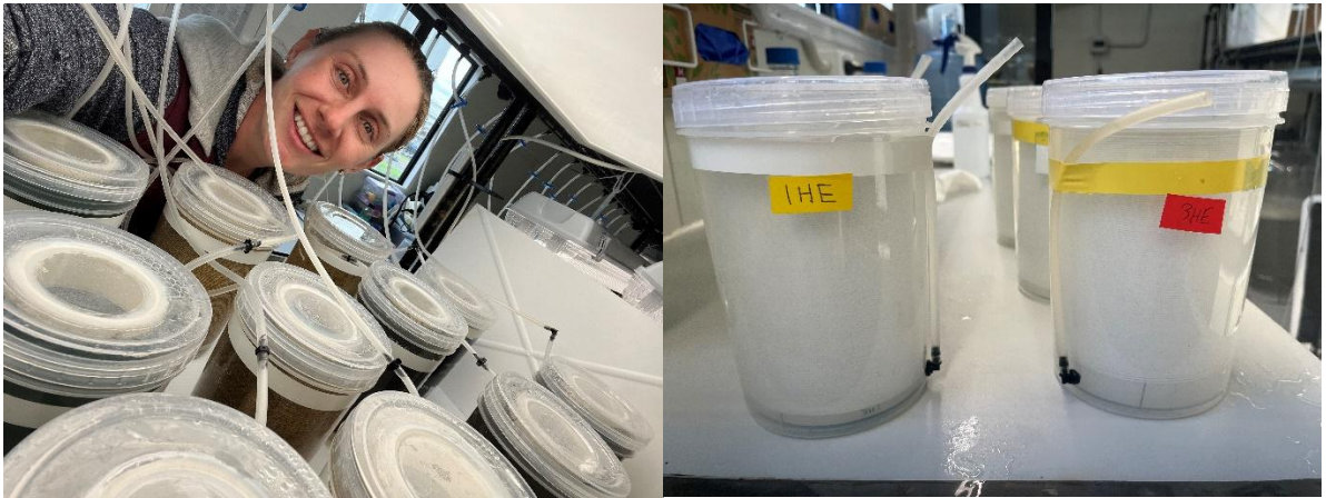
Figure A1. Left: Aerated containers with spools in hatchery with LED lighting from above. Right: Labeled containers with spools at beginning of experiment.
