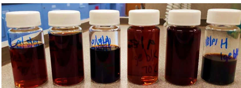
Figure 5.12: Aliquots (20 ml measured on day 14) of 70 °C samples at day 22 showing the difference in evaporation over eight days due to the poor seal created by the lids. Furthermore, the difference in colouration between light (vial 1 and 4), medium (vial 2 and 5) and heavy (vial 3 and 6) samples. Samples labelled from left to right; L_lge, M_lge, H_lge, L_sml, M_sml, H_sml.
