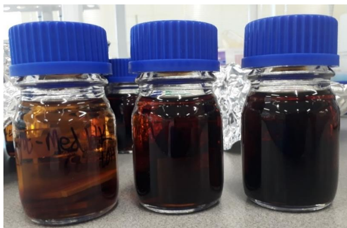
Figure 5.2: Colour change of 65% ethanol solutions with large oak chips (left to right: light, medium and heavy toasting) after one day at 70 °C. The light toasting (left) was a light amber whereas the heavy toasting solution was a dark amber (right).
