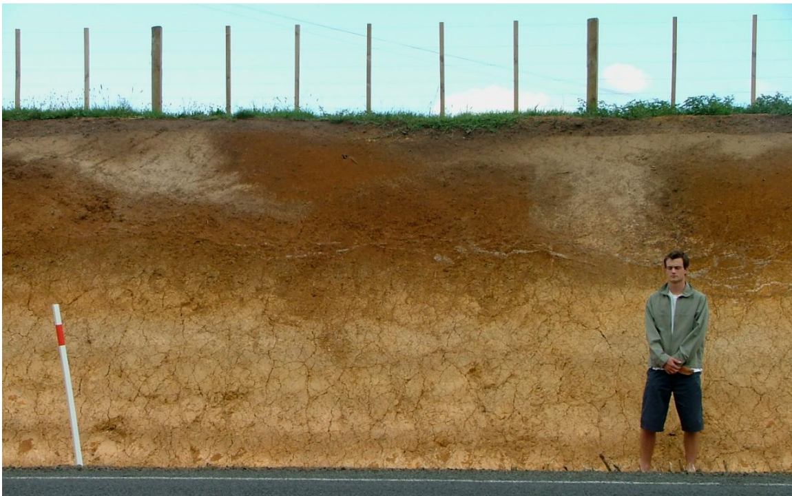
Possible tree overturn features shown up by contrasting colours and textures of pale cover bed tephras (OIS 3-1) and dark reddish-brown soil in weathered upper Hamilton Ash unit H6/7 (OIS 5). Layers of grey (low chroma) clay veins are evident at top of brown unit H5 (OIS 7?) level with Seb’s head. Naike soils occur infrequently where the cover bed is missing. Photo: David Lowe
