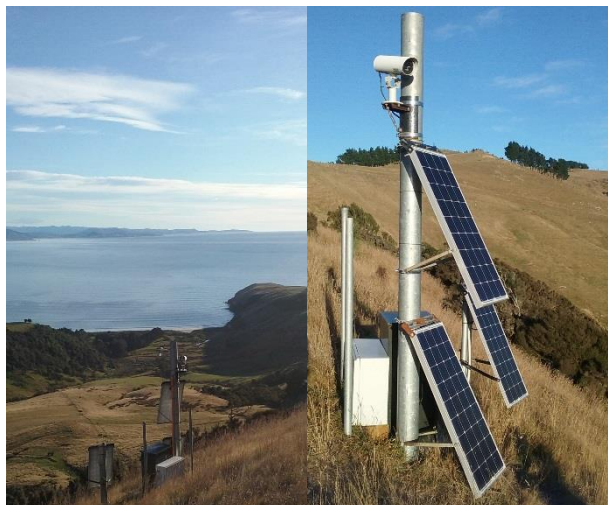
Figure 2. Camera monitoring system installed at Whareakeake at the top of the valley looking down on the surf break along the headland (left image, right hand side).
