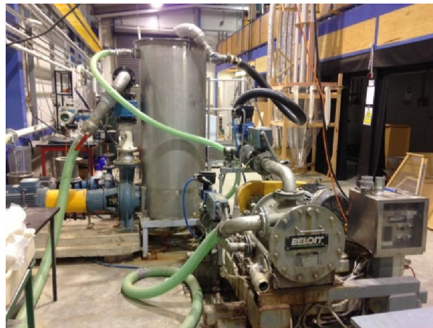
Figure 2.6 Chicken Feather Comminution Apparatus.
