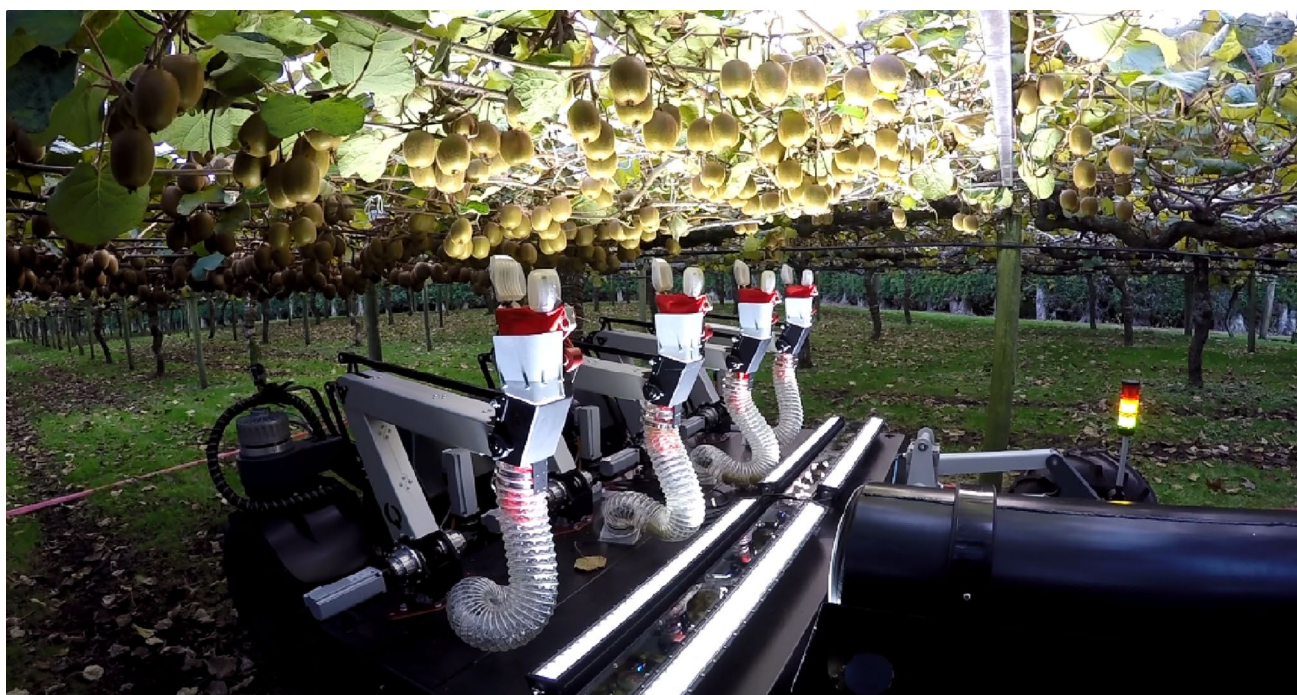
Fig. 1 The kiwifruit harvesting system with four robot modules
