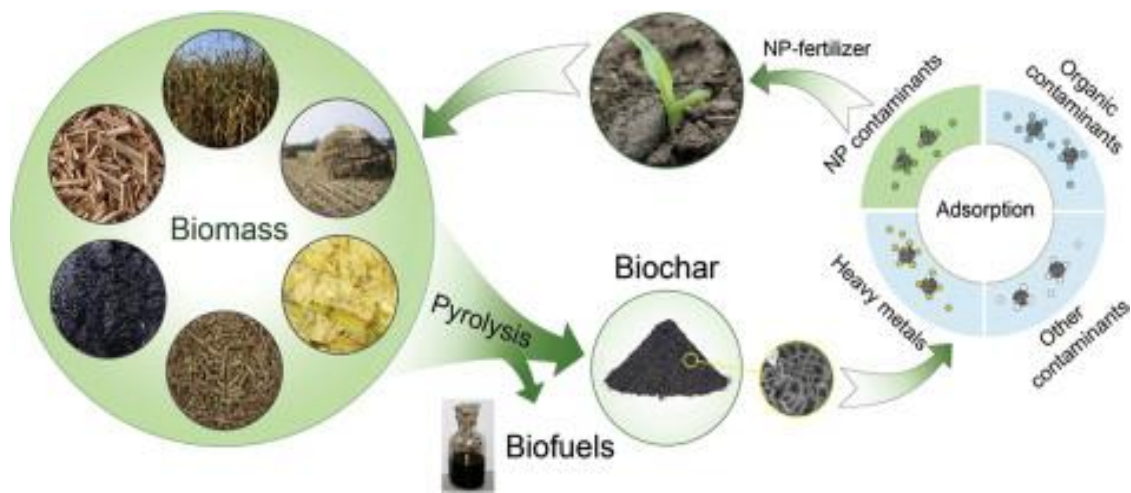
Figure 2-14 Use of biomass to produce biochar and biochar applications (Tan, et al., 2015)
