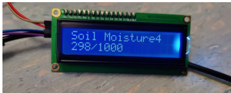
Figure 3-4 Soil moisture reading
