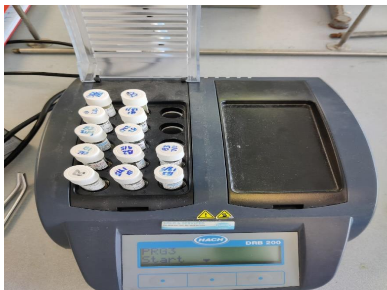
Figure 3-9 Incubation of samples for sugar analysis by digesting at 135 degrees Celsius.
