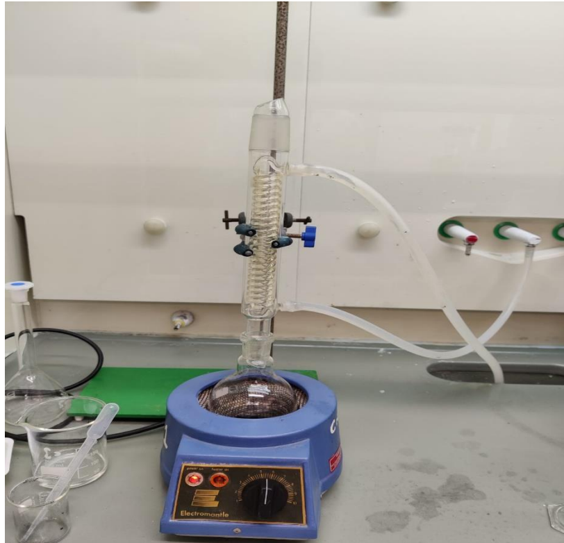
Figure 3-7 Experimental setup for the reflux method for measuring fungal growth
