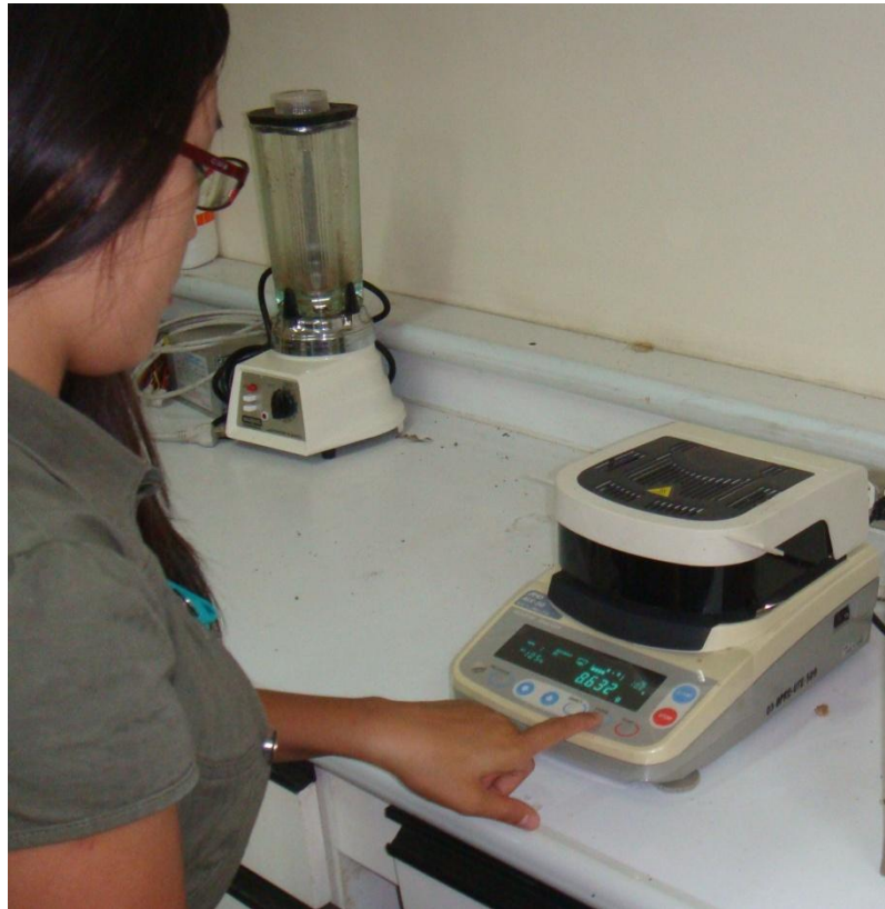
Figure 6.5. Infrared (AD-50) moisture analyzer used in the study
