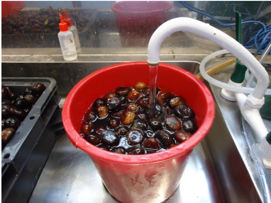
Figure 3.4. Flotation grading method used for chestnut samples
