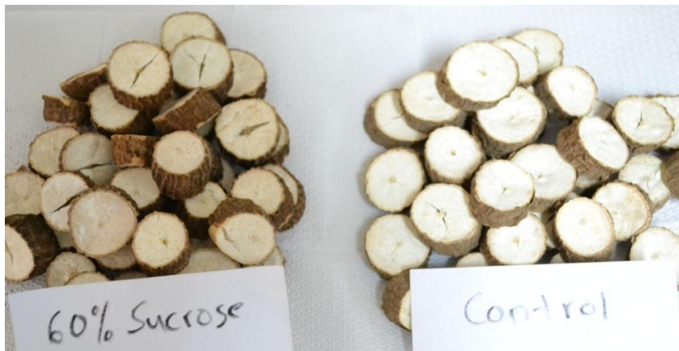
Figure 6.12. Physical comparison of osmosed(60% w/w sucrose) and unosmosed cassava after drying to belt dryer test rig at 70°C drying temperature
