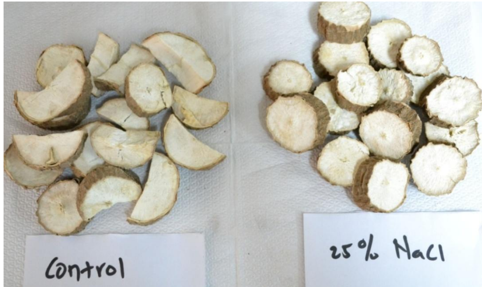
Figure 6.11. Physical comparison of osmosed (25% w/w NaCl) and unosmosed cassava after drying to belt dryer test rig at 70°C drying temperature
