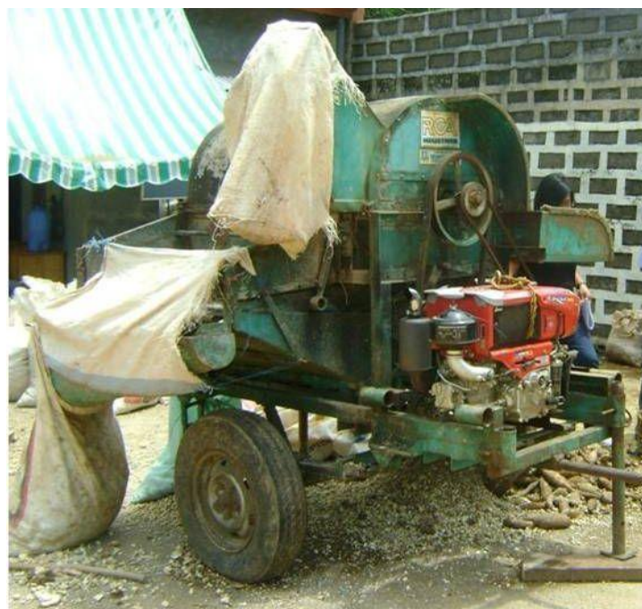
Figure 2.9. Multi-sheller/thresher commonly used as cassava granulator
