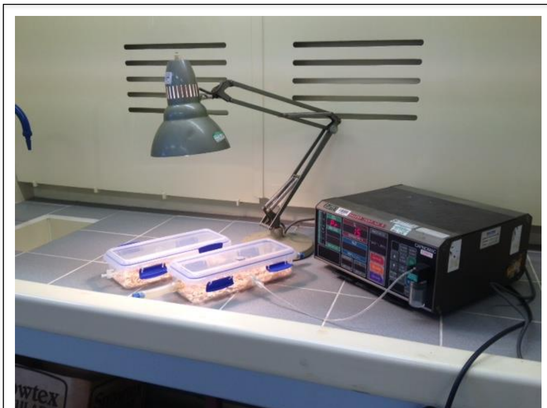
Figure 23: Experimental Design for Delivery of Volatile Anaesthetics Isoflurane and Sevoflurane. Two animal chambers were set up inside the fume hood; one for the t=4 hour control mouse and one for the t=2 hour and t=4 hour treatment mice.
