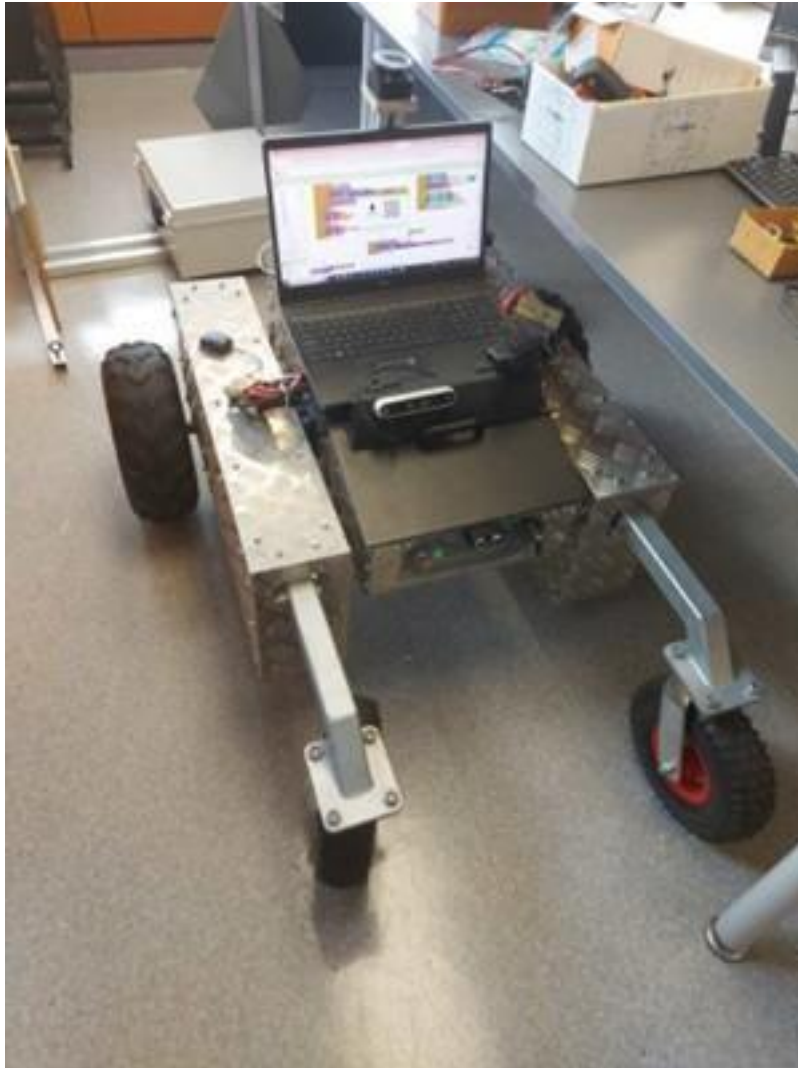
Figure 3.2: Physical assembly of Nicobot showing the chassis, mounted sensors and control hardware. (Source: Pham X. K., 2025)
