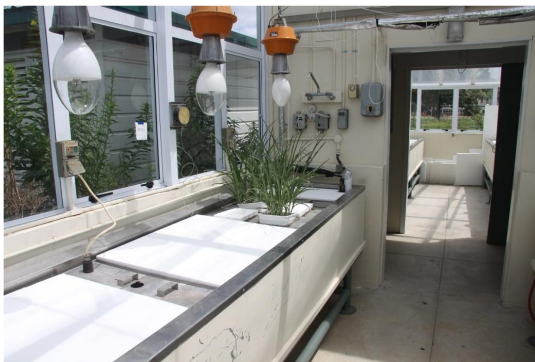
Figure 2.1 The experimental setup. Broom corn millet plants were grown with substrate temperature controlled by floating pots in temperature controlled water baths.
