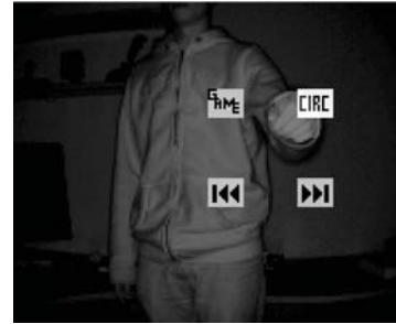
Figure 3: A user interacting with a push button menu by moving their hand in free space.
