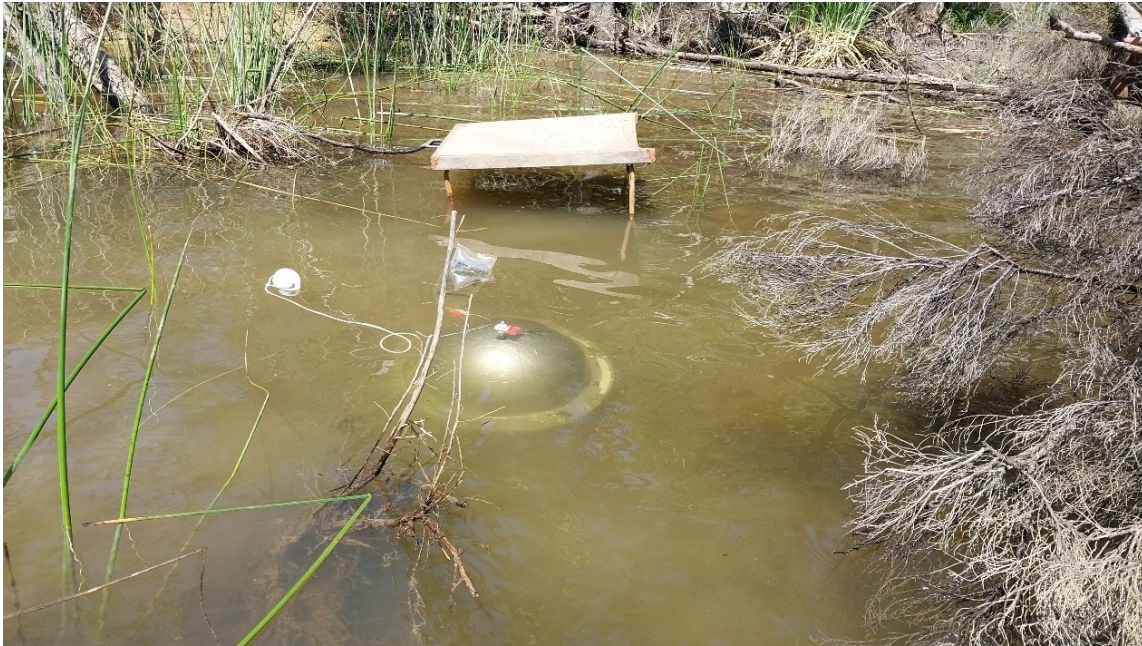
Figure 9. Infiltration chamber used to measure littoral groundwater flux.
