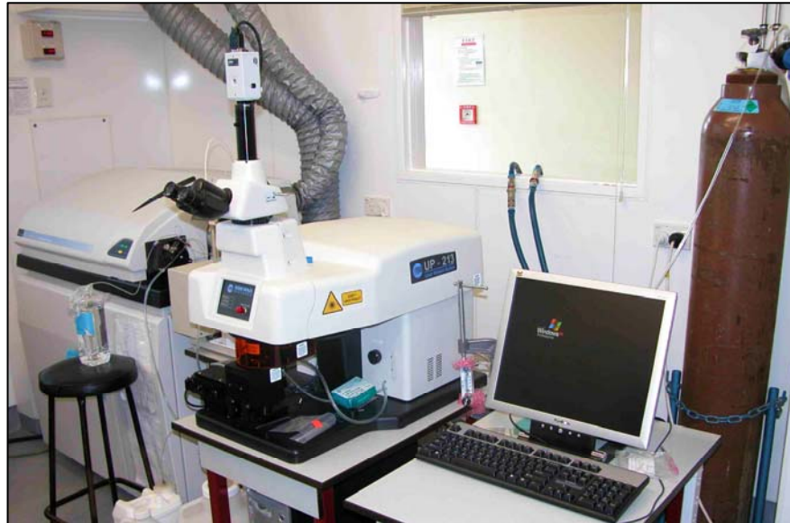
Plate 2.2. Laser ablation inductively-coupled mass spectrometer (ICP-MS) at the University of Waikato.
