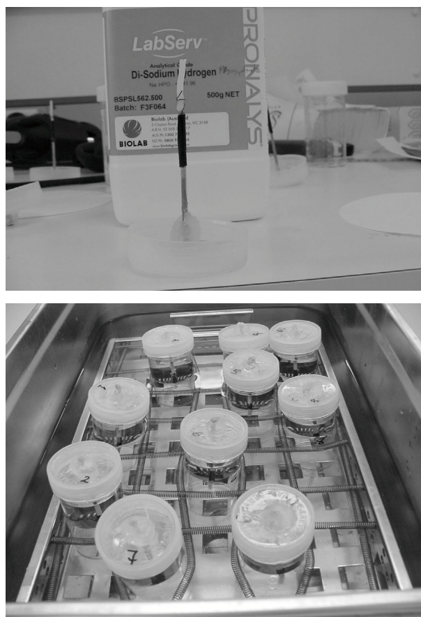
Fig. 3. Upper: Mode of attachment of extruded PEO rods to release media pottle lids. Lower: Pottles in the water bath for testing release of drug from PEO extruded rods into 40% (v/v) ethanol/water.
