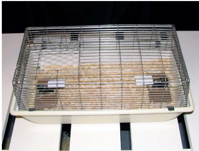
Figure 10.6 A standard rat cage, fitted out for use in the light extinction experiment. One lever was assigned to be the active lever (turning the lights off when pressed), the other the inactive lever (having no effect when pressed). Which lever was the active lever and which was the inactive lever was alternated with each new animal tested).
