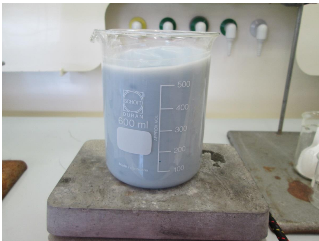
Figure 22: Rapid stirring of the precipitate to encourage oxidation.
