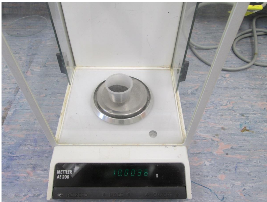
Figure 11: Accurate weighing of a sample of composite material
