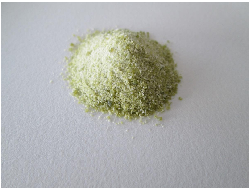
Figure 29: Sodium contaminated precipitated titanium dioxide.
