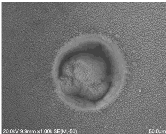
Figure 3.5 Analysis of float glass using a 50 \mu\text{m} spot with 50 % power. The middle of the crater has melted glass present.
