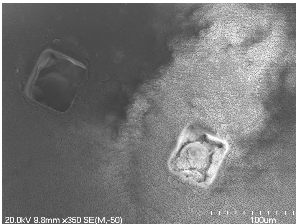
Figure 3.9 Plume from 60 \mu\text{m} spot with 50 % power (right), which is not observed for the 60 \mu\text{m} spot at 90 % power (left).
