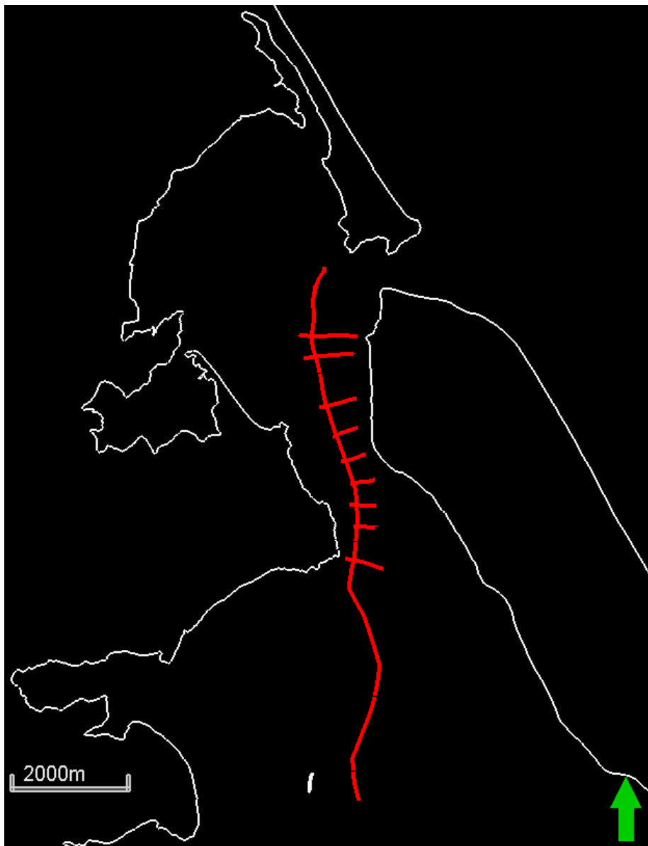
Figure 3.6. Map of seismic lines used to create the structure contour maps and isopach thickness maps of the Seafloor, Horizon A, and Horizon B.
