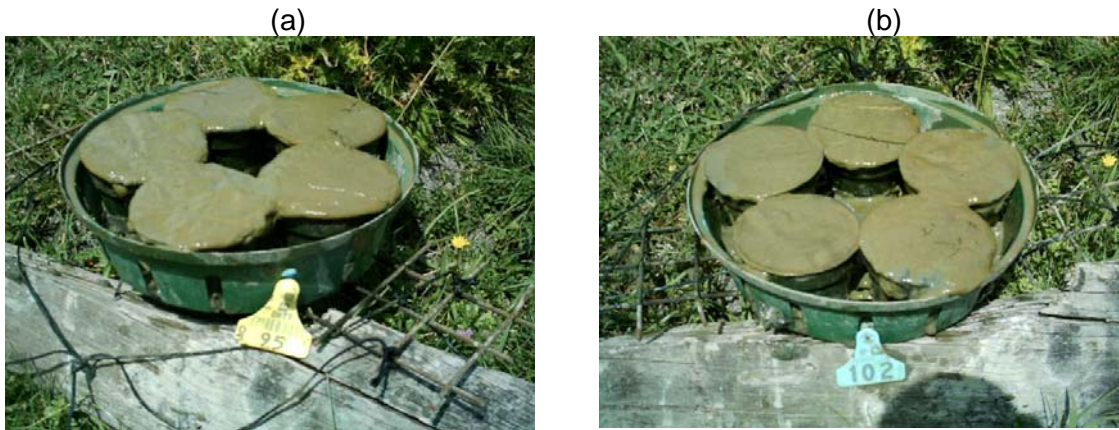
Plate 5: Sedimentation on oospore pots retrieved from the exposed site (a) and the sheltered site (b) at Lake Waikare at Day 90
