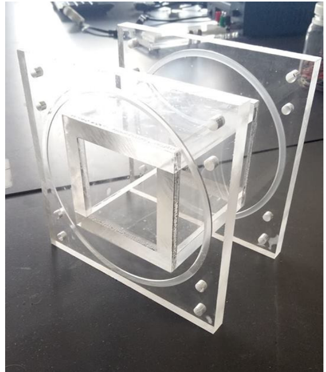
Fig. 9. An example of the larger acoustic waveguide with flanges and alignment pins visible. The component is a short length of plain waveguide, again constructed in transparent acrylic.
